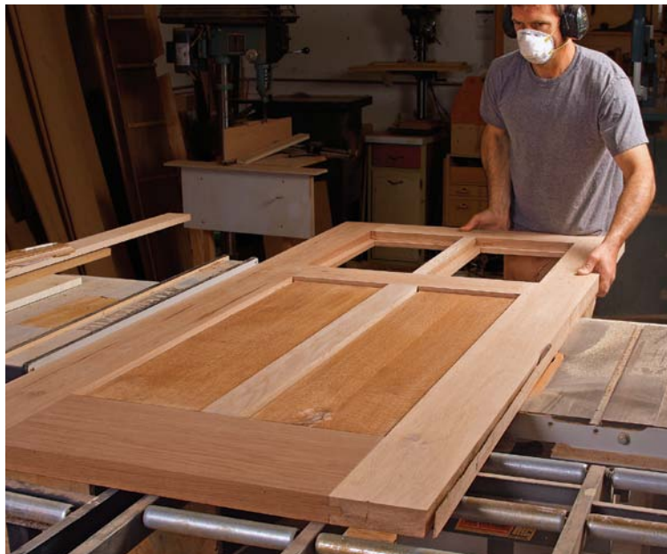
Add the stiles. As a defense against the elements, Finn uses two-part marine epoxy when gluing exterior doors. Once the door is in clamps, you can peg the tenons.
