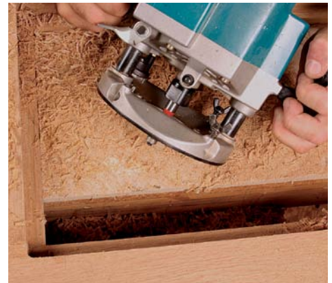
Turn a groove into a rabbet. The glass sits in a rabbet, held with stops. Use a handheld router with a bearing-guided bit to cut away the top of the groove, creating the rabbet.
