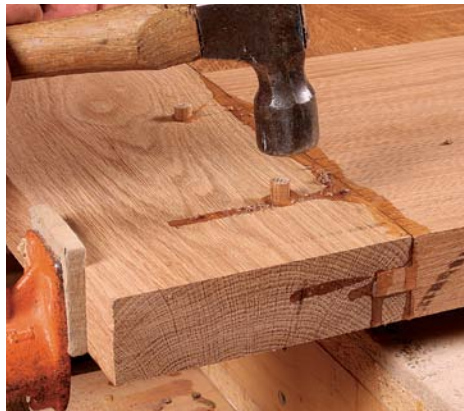
Add the stiles. As a defense against the elements, Finn uses two-part marine epoxy when gluing exterior doors. Once the door is in clamps, you can peg the tenons.
