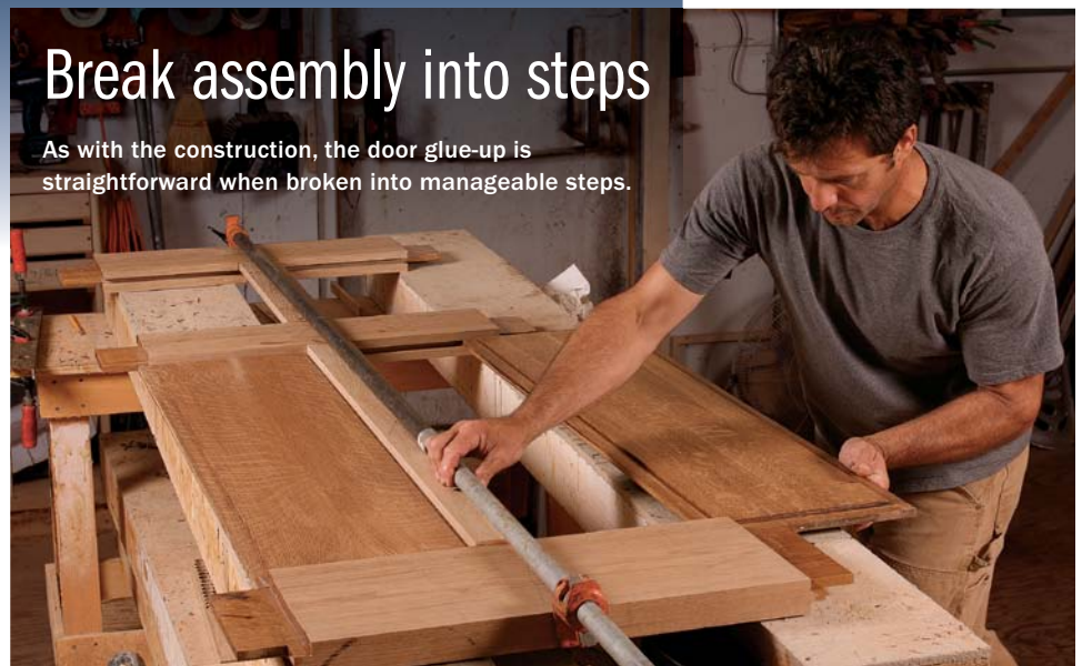
Insert the panels. Prefinish them, or seasonal movement will expose sections of unfinished wood in the rabbets. Then epoxy and clamp the center dividers in place as shown, and slide in the panels.
