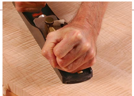
3. HIGHEST ANGLE FOR FIGURED WOOD
