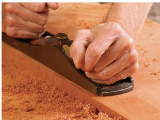
4. TOOTHED BLADE FOR FLATTENING WIDE BOARDS
