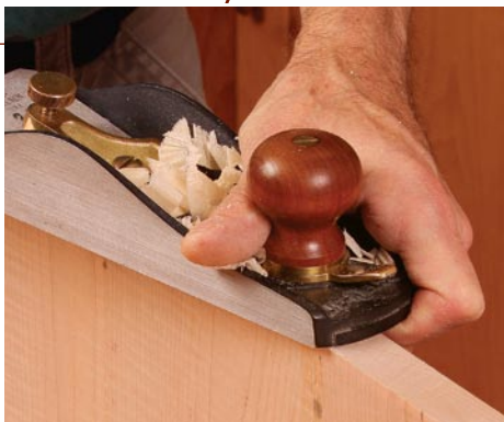
1. STANDARD ANGLE FOR END GRAIN
