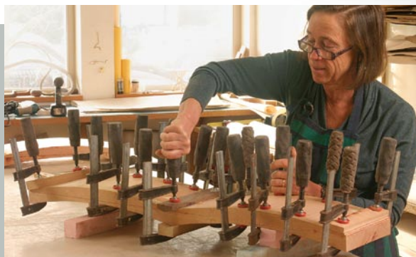
Got clamps? You'll need them now. Ames spaces them 3 in. apart and uses shaped cauls to get pressure into the valley where the offcuts meet.
