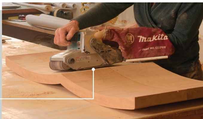
And smooth the seat. When gluing, Ames aligns the two halves simply by sight and feel. Afterward, she again sands across the grain (right). The platen for the top side needs only a slight curve. After sanding, Ames uses a card scraper.
