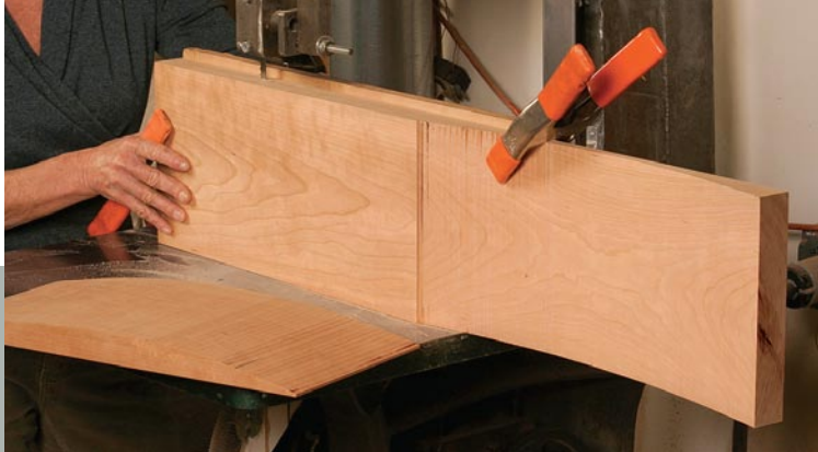
Get help to hold the board upright. Ames clamps the board to an L-shaped plywood support to keep it parallel to the blade, which minimizes the amount of sanding needed afterward.
