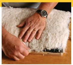
**Cover the edging.** The third or fourth piece of batting should reach the contoured edges of the rubberized horsehair.
