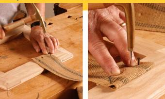
**Tack and fold.** Cut off a strip of webbing about 6 in. longer than the width of the frame. Tack down one end just inside the bevel using five #6 tacks, staggering the tacks slightly to avoid splitting the wood. Fold the webbing over the tacked end to create a double layer, and tack this down as well, interspacing the tacks with the first set.
