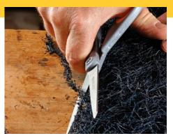
**Tack and trim.** Apply a layer of rubberized horsehair padding following the outline of the seat. Secure the horsehair with two #3 tacks per side and then use scissors to slightly round over the top edges.
