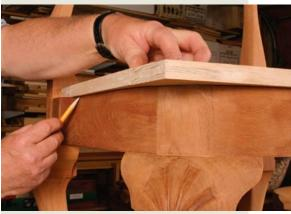
**Matching curves.** Transfer the curve of the chair rails to the underside of the slip-seat frame.
