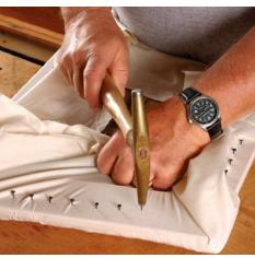
**Stretch and tack lightly.** Stretch the muslin, making sure there are no wrinkles along the edge of the frame. Apply three tacks, working out from the center. Don't drive them home. Go around the frame, working evenly out from the center of each side, keeping the muslin evenly stretched and wrinkle-free.
