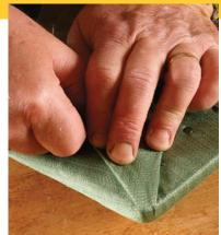
**Pull to remove wrinkles.** Ensure that wrinkles are eliminated, particularly at the corners.
