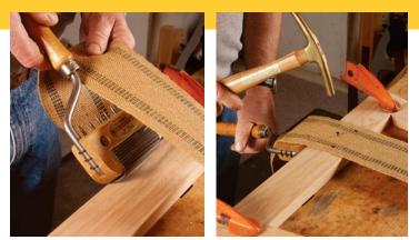
**Stretch and tack.** Stretch the webbing across the frame using a webbing stretcher. The webbing should be tight but not enough to distort the frame. Anchor this end of the webbing in a similar way with another double row of tacks. The magnetic-tipped hammer allows you to pick up the tacks while one hand holds the stretcher.
