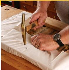
**Tack lightly.** Cut the muslin so it extends 6 in. beyond the frame on all sides. Lightly stretch it over the padding and secure it with one #3 tack centered on the bottom of each frame piece.
