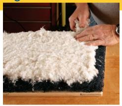
**Move outward.** Add progressively larger squares of <sup>1</sup>/<sub>2</sub>-in.-thick batting. Pull the edges to feather them down onto the rubberized horsehair.
