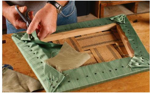
Trim the excess. Cut away surplus fabric to leave the underside of the frame as flat as possible.
