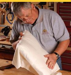
**Check the fit and finish.** Look at the seat, and sit on it to determine if cotton batting needs to be added or removed.
