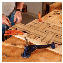
**Over and under.** When attaching the side-toside webbing, go over and under the front-toback webbing to create a weave.
