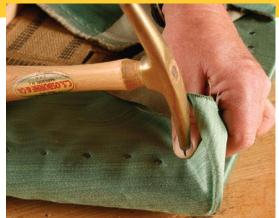
**The top layer.** Don't stretch the finish fabric as tightly as the muslin. Use longer #4 tacks, and make sure the weave and any pattern are oriented correctly.
