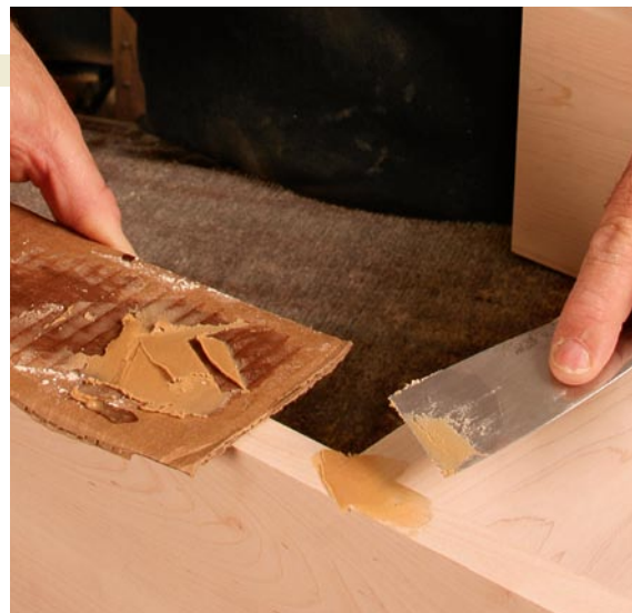
Fill the gap. Use a putty knife to force the filler into the open joint. The color difference will disappear when the filler dries and finish is applied.
