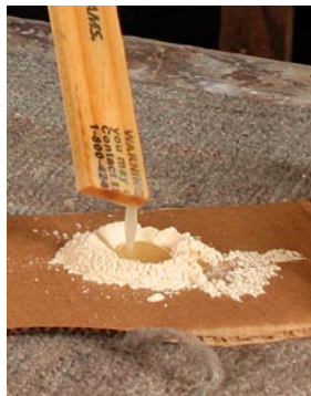
Shopmade filler. Save sanding dust from your project and mix it with either lacquer or shellac to form a stiff filler.
