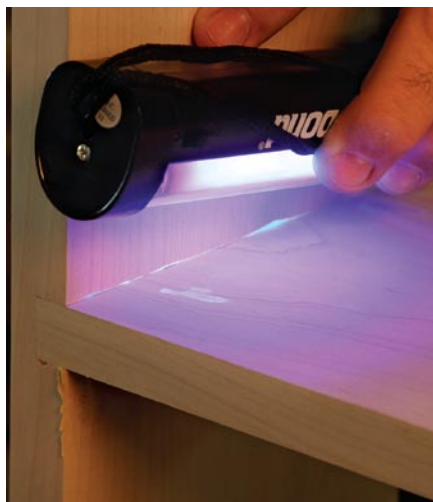
Try fluorescent glue. A black light will reveal any traces left on the surface.
