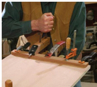
Glue blocks beef up the corners. The glue blocks, attached to the top and bottom of each side, increase strength against racking.
