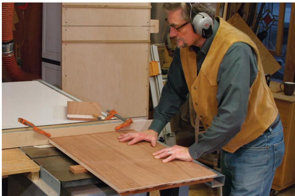
Use a dado set to rabbet the sides. Bury the blade in a sacrificial fence to dial in the width. Place an offcut from the glue-block stock under the workpiece to stabilize it.
