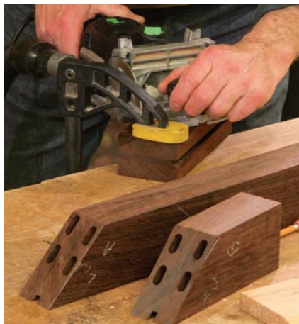
Tenons brace the corners. Each miter gets four slip tenons (left). Glue up the mitered feet first (above), then attach them to the stretcher assembly (below).
