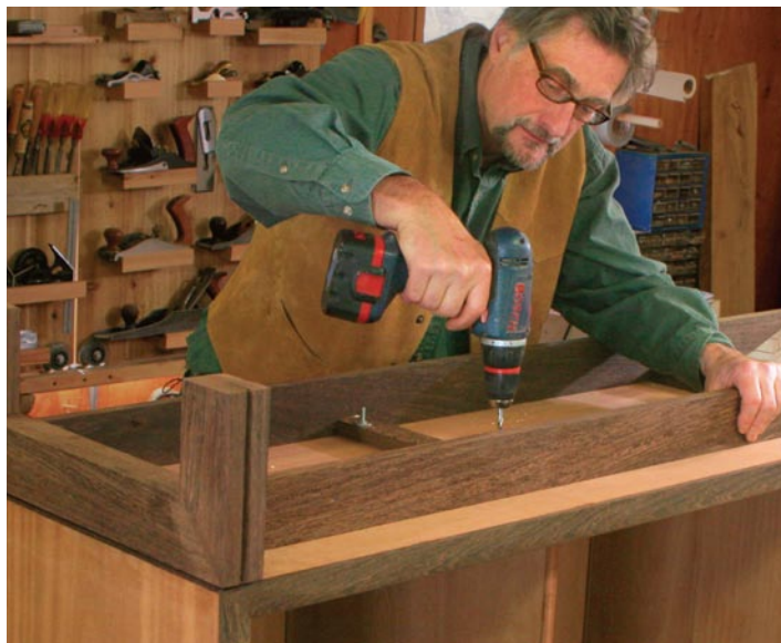
Bolt the base to the case. Drill clearance holes through the base and bottom of the case, then bolt the assembly in place.
