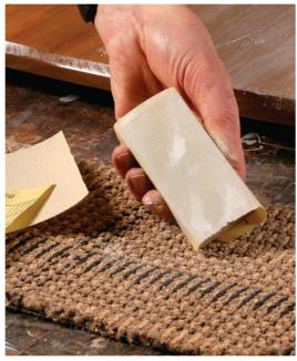
How to sand efficiently. Fine P320-grit sandpaper has a short life span, so move to a fresh piece as soon as it stops cutting. A quick way to unclog the sandpaper is to wipe it on a remnant of carpet. Stiff and coarse weaves work best. Don't try to sand out every small depression in the surface.
