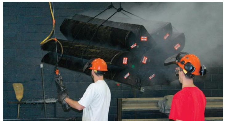
Kept wet. Sprinklers keep the logs wet and prevent them from drying out and checking.
