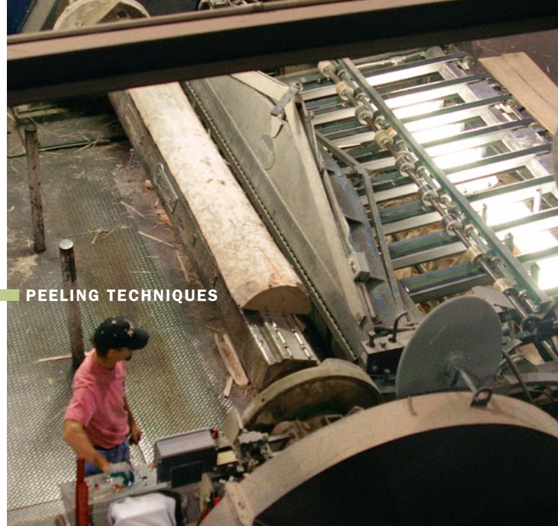
Round and round. Rotary-cutting, or peeling, produces wider sheets from smaller logs and is also used for certain figured veneers.
