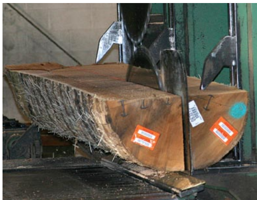
Hand-picked. The logs arrive at the veneer mill already marked with a unique barcode. Metal “S” irons or plastic “I” clips minimize end splits.
