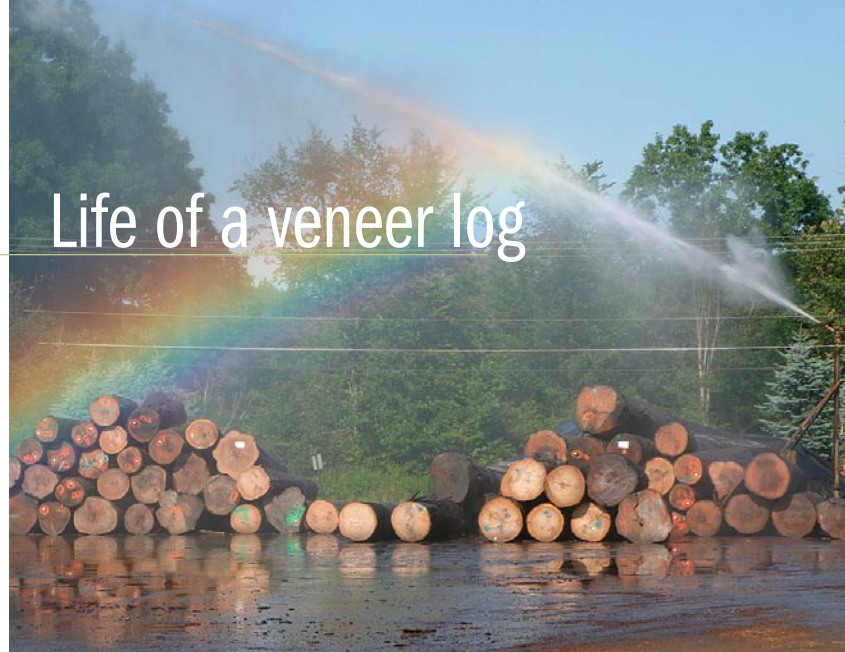
Kept wet. Sprinklers keep the logs wet and prevent them from drying out and checking.
