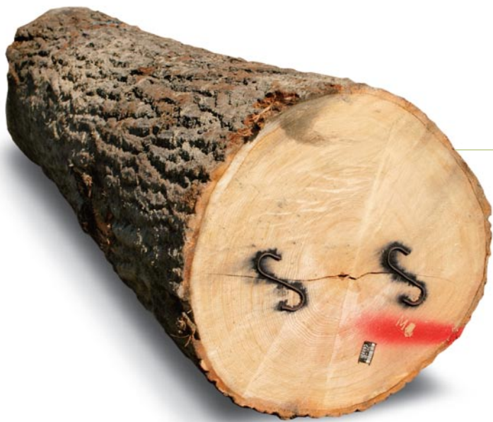
Hand-picked. The logs arrive at the veneer mill already marked with a unique barcode. Metal “S” irons or plastic “I” clips minimize end splits.
