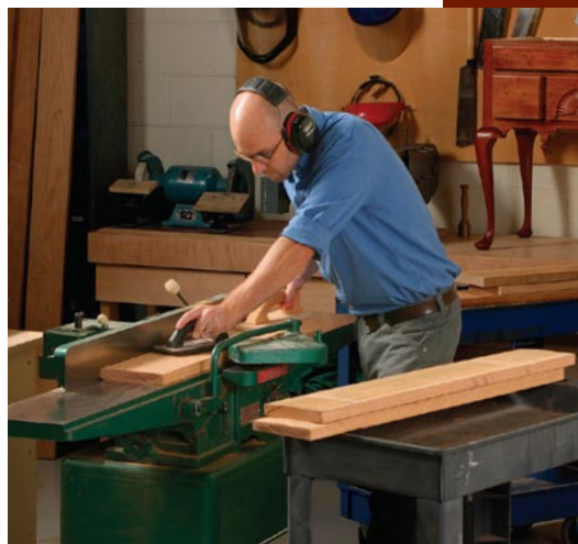
Faces, but no edges. Lipp starts by flattening a face, but doesn't then straighten an edge. It's not always possible to feed edge grain into the jointer properly when only one face is jointed.
