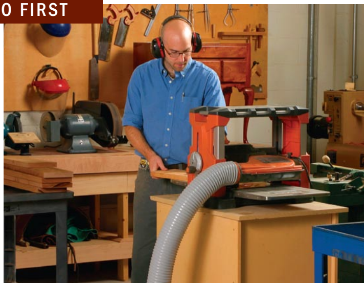
Plane second face flat. When the board is about 90% flat, begin to flip it end for end after each pass. That keeps the grain running in the right direction as you take equal amounts off each face, which relieves internal tensions evenly and minimizes how much the board will cup afterward.
