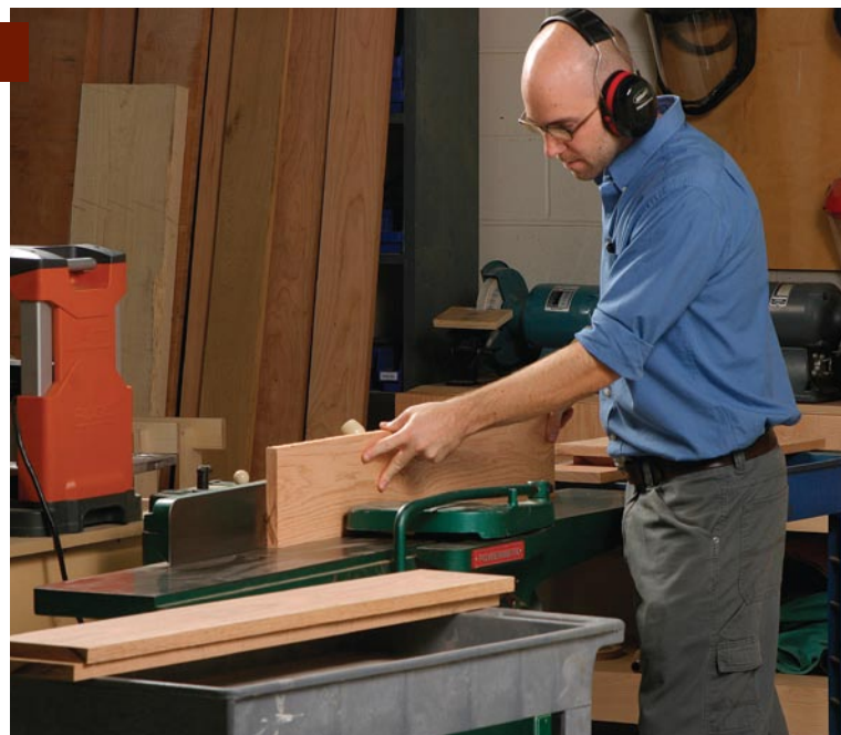
Right edge, right direction. Joint the concave side for stability. Both faces are flat and straight so you can flip the board either way to avoid tearout.
