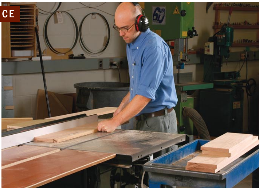
Straight from cart to blade. For safer ripping on the tablesaw, a board must have a straight edge to run against the fence. Also, use a push stick on narrow boards.
