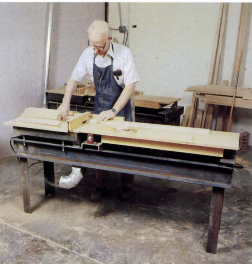
T.H. Ralph's sliding-table crosscut saw has 9-in. travel and will saw stock up to 2¼ in. thick. The Thomson linear-motion bearings, visible in the photo at near right, ride on a 1¼-in. precision-ground shaft mounted in a pair of steel supports. The sliding table's outboard end rolls on a wheel cannibalized from garage-door hardware. Its bearing surface (photo at far right) is a piece of heavy angle iron that can be raised or lowered to square the table to the blade in the horizontal plane.
