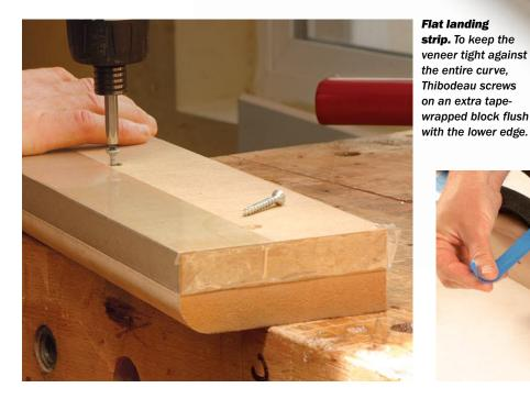
Deco chess table, or downward as in crown molding. I laminate a stack of MDF for the substrate. I use the method described in *FWW* #168 ("Cutting Coves on the Tablesaw") to lay out and cut the coves. They usually need some sanding afterward to smooth the tablesaw cut. I don't use a vacuum bag to press large coves; I find it easier to clamp them manually. Before veneering the cove in this case, I veneered the flat edges adjoining it. Those are also easy to veneer with clamps and cauls.
