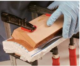
Flip check. Clamp the assembly firmly and uniformly along its length. Turn over the glueup and check the squeeze-out to be sure all of the edges are clamped. The white foam will continue to compress, so come back in 10 minutes to retighten the clamps.
