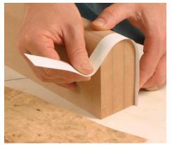
**Measure for the veneer.** Make the workpiece extra wide at this point, and use a flexible ruler or a strip of paper to see how much veneer is needed. Cut the veneer about  $\frac{1}{2}$  in. short to allow it to expand when it hits the yellow glue.
