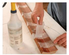
**Remove the tape.** Thibodeau uses thin, wide gum tape to join sections and reinforce curves. It comes off easily when dampened and allowed to soften.
