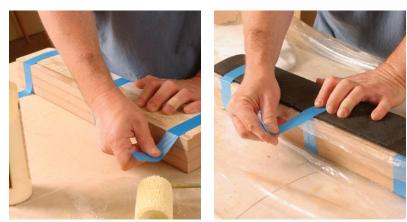
**Lock it down.** After applying glue, tape down the veneer (left) to keep it from sliding around. Then tape down the layer of plastic sheeting and neoprene (right).
