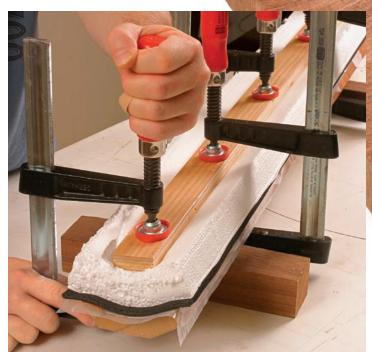
Mix and spread glue. Use ureaformaldehyde glue for coves. Spread it evenly on the substrate using a roller designed for adhesives. Wait a few minutes for some to be absorbed, and then apply a thin second coat.
