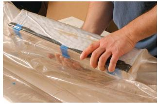
**Press and wrap.** Thibodeau adds a layer of white breather cloth to help the airflow. He smooths the wrinkles and wraps the bag tightly around the bottom corners as the air escapes.
