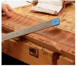
**Two ways to trim.** If the veneer is sticking straight out, a flush-trimming bit works great (left). But if the veneer bag has flattened the edge, use a machinist's "float" to file the corner (right) until the excess drops away, then sand it flush with a hard block and P100-grit paper.
