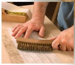
**Tape outside curves.** The wet gum tape prevents splintering and keeps the veneer flexible. Burnish the tape with a brass-bristle brush to improve its bond. Cover the veneer temporarily with a piece of MDF to keep it flat and moist.
