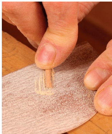
Flatten the dowels to create a perfect fit. Sand a flat into each dowel and then insert it, flat side against the top of the frame, until hand tight.
