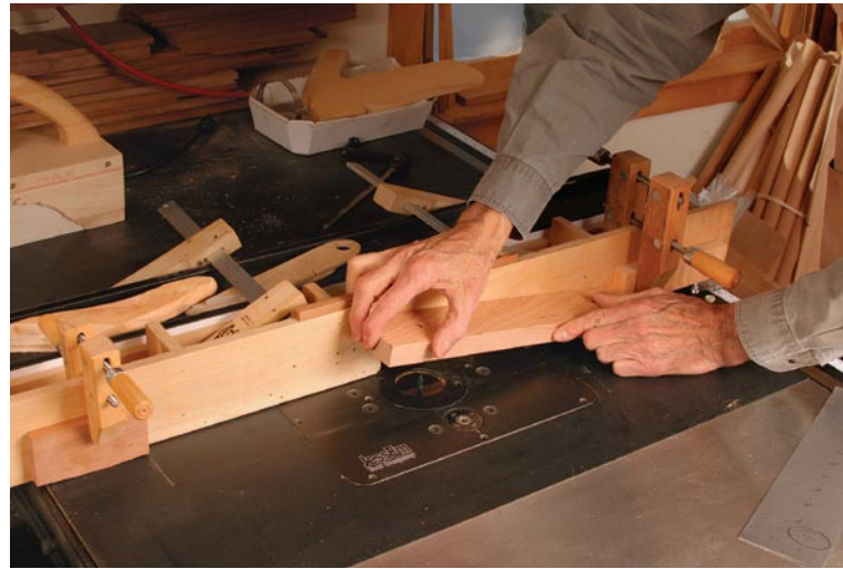
Stopped grooves in the top and bottom. With two stop blocks clamped to the fence so that the bit lines up in the mortise holes at each end, pivot down into the first hole with the router running, run the groove, and lift the workpiece out of the second hole.
