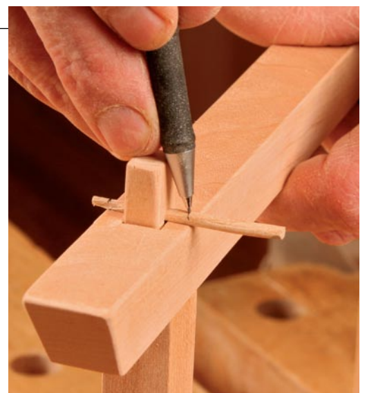
The final cut. Mark the dowels and cut them to length, flush with the sides of the frame.
