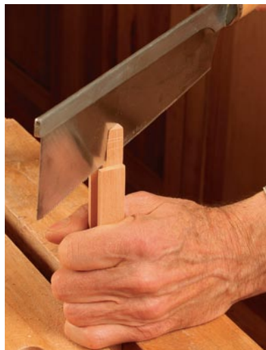
Lower tenons are wedged. Saw a diagonal kerf in the bottom tenons. When the wedges are tapped in, the tenons will spread in all directions.
