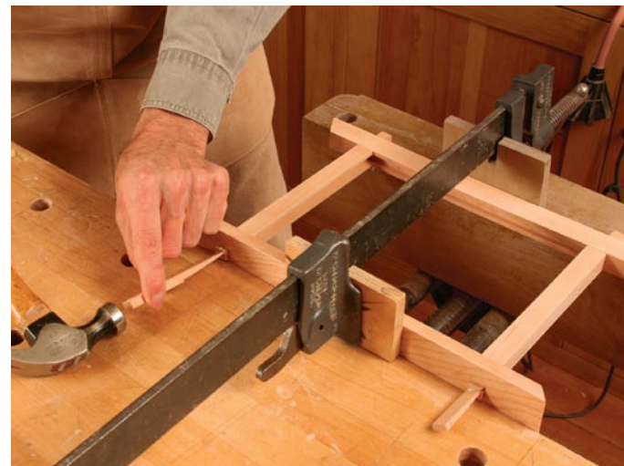
Tap in wedges. Glue the sides into the bottom, set the top in place for clamping, glue the wedges, and tap them into place. Saw the tenons and wedges flush, and then smooth the bottom with a block plane.
