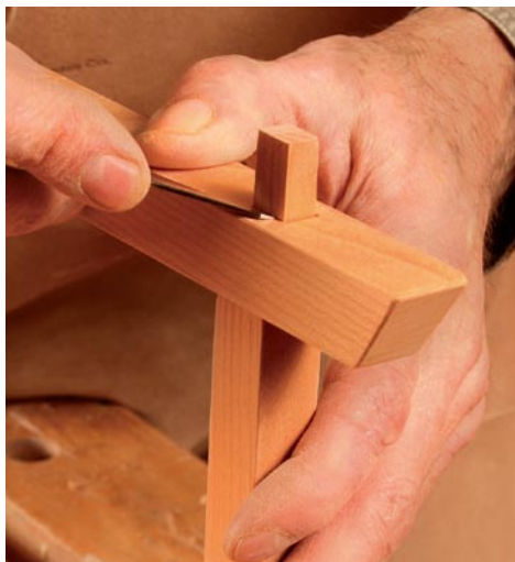
Dowels secure the top. Dry-fit the frame to mark for the dowels. Mark the point where the tenon protrudes. Drill a hole at that point, overlapping the knife mark by about \frac{1}{32} in.
