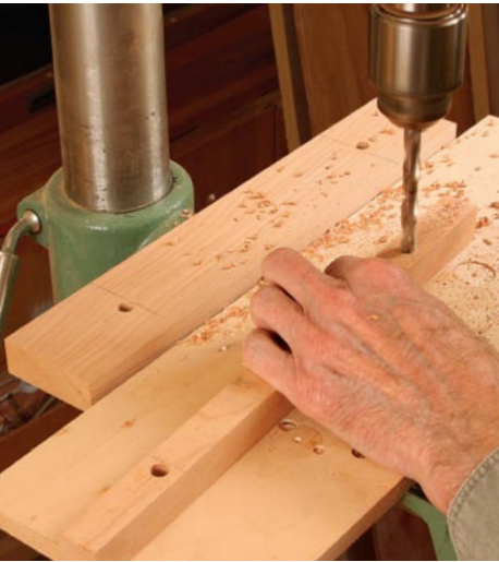
Start on the drill press. Drill through the top and bottom, centering the mortise holes in the stock.
