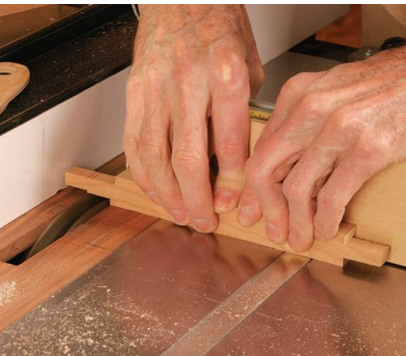
Quick and easy tenons. Using a dado set, miter gauge, and the rip fence as a stop, form the tenons on the side pieces.
