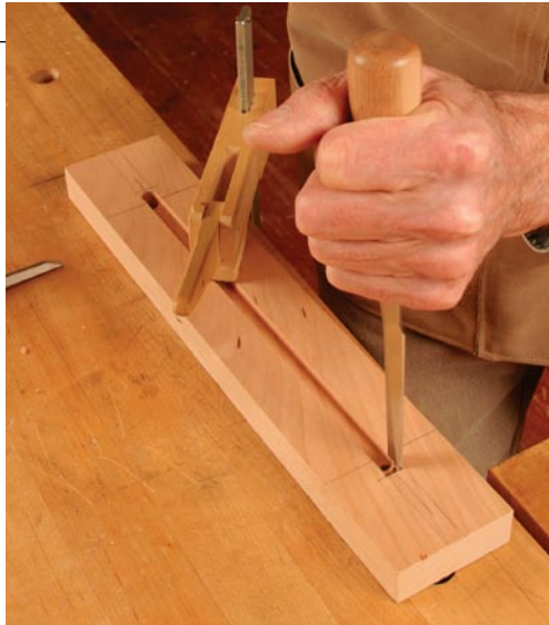
Chisel the mortises square. Now square up the mortise holes all the way through the top and bottom pieces.
