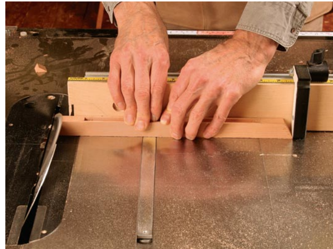
Angle the ends, too. With the table saw blade still tilted from the bevel, use a miter sled and cut angles on the ends of the top and bottom.
