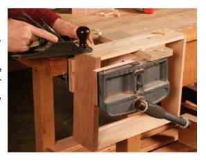
and racking the vise, position the stock between the vise screw and a guide bar, as low in the jaw as possible. The farther up from the jaws the operation gets, the greater the potential for losing control.
