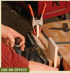
Match its thickness to your workpiece to prevent the front jaw from pivoting. A spring clamp keeps the scrap from falling before the vise is closed.
