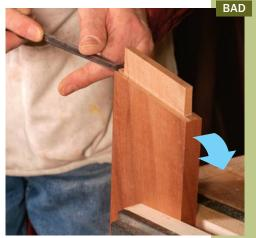
Even wide stock can slip. It's natural to place the broadest faces against the jaws (left), but clamping on the edges still provides enough pressure to hold the work securely (below). Now the piece is braced against the force of the cut and won't slip.
