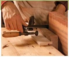
**Just add clamps.** To hold the free end of a long board for edge-planing, secure the crosspiece to the bench and the workpiece to the block. The setup also works for wide boards.
