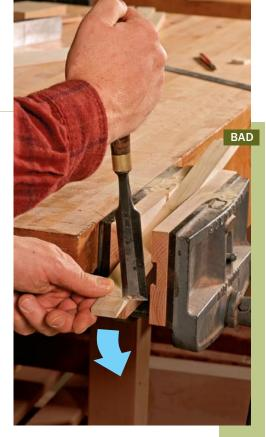
This is dangerous. With no support underneath, the workpiece and chisel can slip under downward pressure (left). Place a support block in the vise underneath the work (below).
