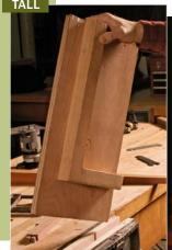
A fixture for legs. Latta uses a panel with an L-shaped bracket to support long work vertically (above). The fixture's top provides a bearing surface for the router when cutting dovetail mortises in the top of a table leg (right). The bottom of the L provides an index for clamping into the vise.
