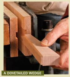
Latta's anti-racking wedge won't fall out because it slides on a dovetailed key routed into the inner jaw. Slide the wedge farther in to accommodate thicker stock.
