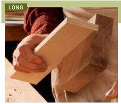
**Fixture helps hold wide or long boards.** The block is as thick as the vise's rear jaw. Leave the crosspiece long to accommodate a clamp.
