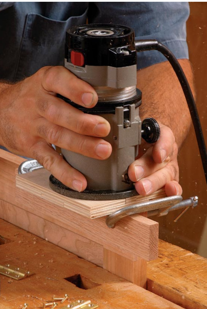
Rout the door mortise. Don't pull the router off the jig until the bit has stopped spinning. If you do, the bit could cut into the template opening and ruin it.
