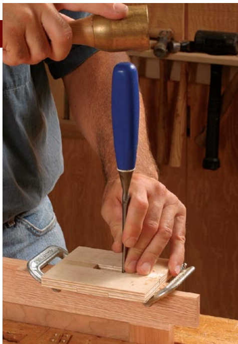
The jig squares corners, too. The square opening makes a perfect chisel guide. Remove the template to pare away the waste (below).
