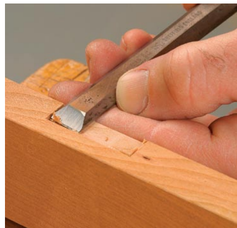
The jig squares corners, too. The square opening makes a perfect chisel guide. Remove the template to pare away the waste (below).
