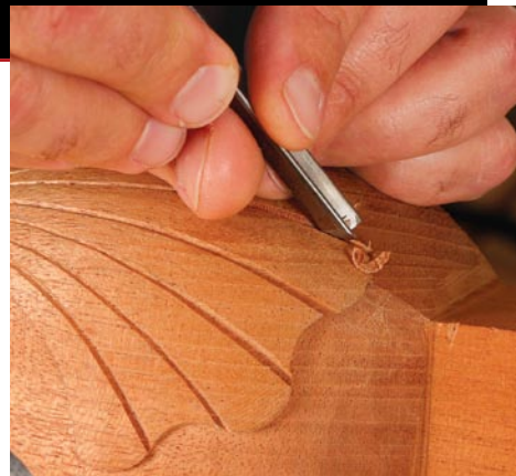
Outline the lobes. Establish each of the lobes by using a V-parting tool to cut along the lines drawn earlier.
