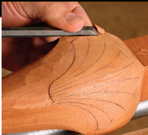
Carve the area around the shell. Bird uses a paring chisel to remove material around the shell until it sits about \frac{1}{16} in. above the leg.
