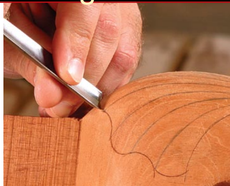
Incise the shell perimeter. Use gouges to incise the entire perimeter of the shell.
