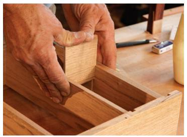
**Install the divider and back.** Press the divider into place (above) and plane it flush after the glue has dried. The back consists of three shiplapped boards that are beveled to fit the grooves in the case sides and top. Slide them in from the bottom (right) and nail them to the shelves.
