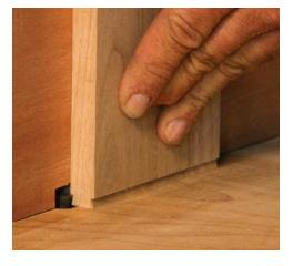
A few more steps. After grooving the sides and top for the back panel, rabbet the sides for the face frame (right).
