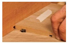
Rout the dovetail slots and keys. With the case sides still taped together, set a dovetail bit at the same height as the dadoes and rout the slots (above). Without moving the bit, adjust the fence to cut the keys in the case top and bottom (right).
