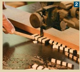
Rip the other edge. Rip the crosscuts into <sup>3</sup>/<sub>4e-in.-thick</sub> strips on the bandsaw. Clean up the saw marks with a block plane.
