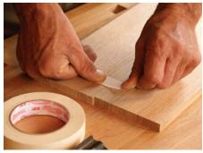
Perfect alignment, guaranteed. To be sure all the dadoes and dovetail slots align perfectly, tape the sides together (above) when you cut the joints. Start by cutting the sides to length on the tablesaw, then install a dado blade to cut the shelf dadoes (right). Cut the same 5/16-in.-wide dadoes at the sliding-dovetail locations. This will clear a path for the dovetail bit (below).
