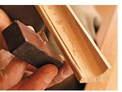
Add the molding. The "ears" that extend beyond the dovetailed case top provide a convenient clamping surface for the molding. A bead, cut with a scratch stock (above), is a place transition for the handling.
