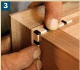
Start at a corner. Glue the banding in place one segment at a time. Rub a block of wood over the banding (right) to seat it in place. No clamping is necessary.
