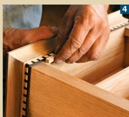
Finish off the bottom. Hack added a thin strip of ebony to the bottom edge of the banding to create a pleasing border. Again, simply rub it on to attach it.
