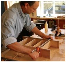
**Shelves first.** Start by gluing the shelves into their dadoes and clamping them in place (above). Slide the case top and bottom into place from the rear (right).
