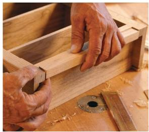
**Face frame comes next.** Check the fit of the face-frame stiles, and then glue them into their rabbets (left). Complete the face frame simply by gluing rails to the case top and bottom (right).
