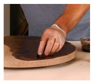
**Apply dye liberally.** Use a folded piece of cloth or paper towel to dye the wood (above). After a minute or two, wipe off the surplus with a clean cloth (right).
