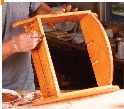
**Reversible color.** When applied to a sealed surface, the gel stain becomes a glaze and can be wiped on and off until the appearance is just the way you want it.
