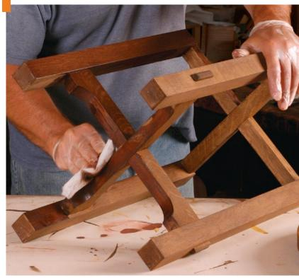
Wipe on, wipe off. Applied straight to the dyed wood, the gel stain packs the pores and emphasizes the grain pattern of the white oak.
