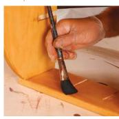
**Yellow adds depth.** Wipe the sealed pine with the yellow dye (left). Apply a 2-lb. cut of dewaxed shellac (right) to seal the dye before using the gel stain as a glaze.
