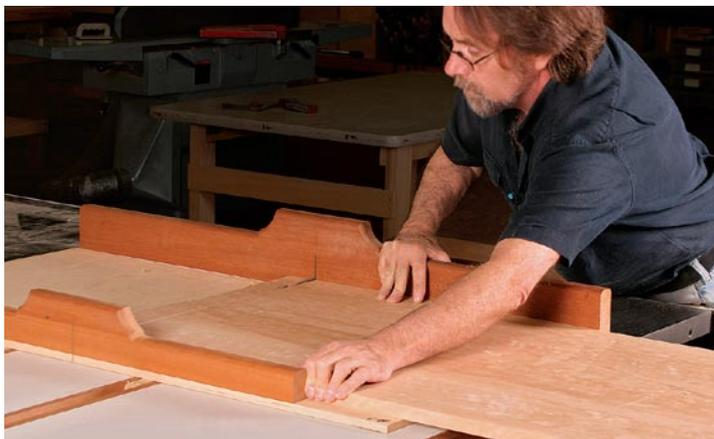
**Does it fit your sled?** If your tabletop is narrow enough, use a crosscut sled to cut it to length quickly and safely.
