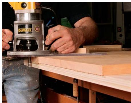
**Use a router for wide tabletops.** If the top is too big to be crosscut safely on the table saw, lay out the cut, and use a jigsaw or a circular saw to cut just outside the line (above left). Then use a bearing-guided router bit riding against a straightedge to trim the waste up to the line (above right). Whichever way you cut the top to length, use a sanding block, a low-angle block plane, or better still a low-angle smoother to clean up the ends of the tabletop (below).
