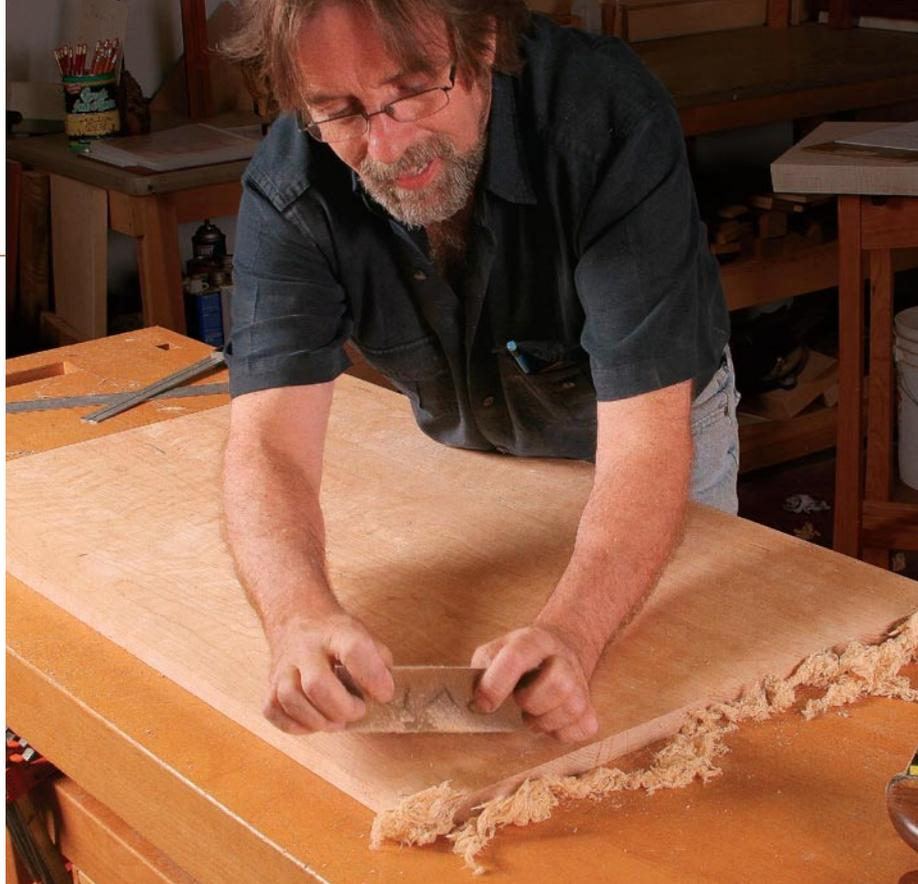
out any marks left from the tablesaw or the router. End grain is tough to plane, so take very light cuts and skew the plane. A little furniture wax on the sole of the plane also will help it cut smoothly. To avoid tearing out the long grain of the far edge, stop planing an inch or two before the end and then come at it from the opposite side. Now wrap a piece of P320- or P400-grit sandpaper around a cork sanding block and, with a few strokes, you will have ends that feel like glass.
