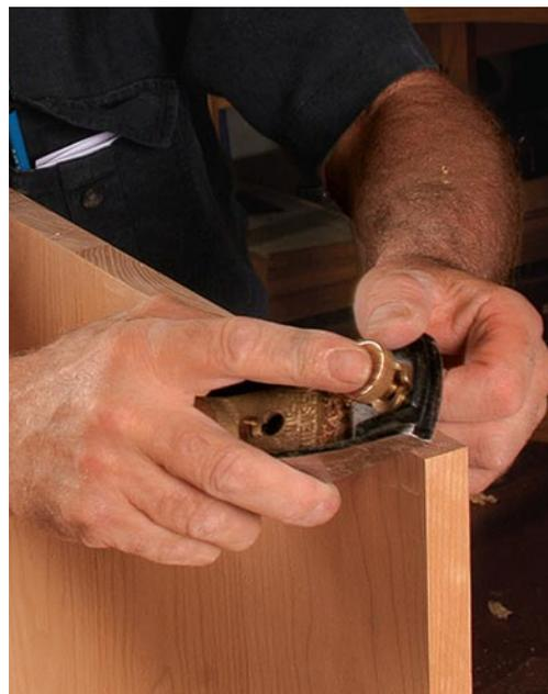
**Break the edges.** Use a block plane to create small chamfers on all the edges. This lessens the chances of the top being damaged, makes applying a finish much easier, and feels better to the touch.
