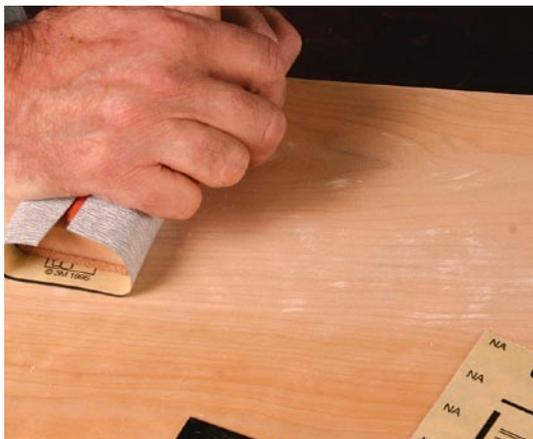
**Tearout revealed.** It can be hard to see minor tearout left by handplanes. Lightly sand the surface with P320- or P400-grit paper to highlight the torn-out areas (above). A sharp card scraper quickly removes any tearout you find (right), but be careful not to create hollows.
