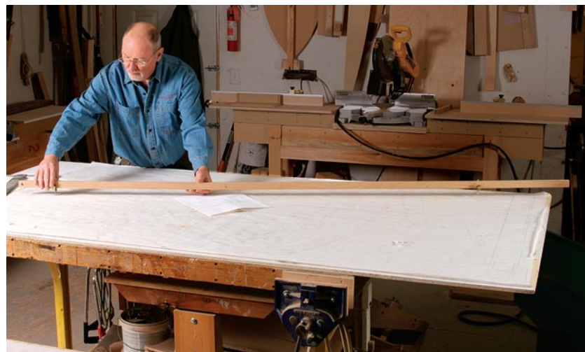
Supersize. Heavy-duty beam compasses are attached to thicker stock to draw ultralarge-diameter arcs.
