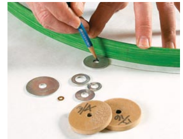
Parallel. To add thickness to a curved part such as a drawer front, you need to draw two lines that are evenly spaced apart. Simple metal washers or shopmade MDF versions work well.
