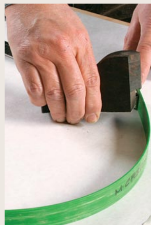
Heavy helping hands. It's tough to hold the bow and trace a line at the same time. If you don't have a helper, use spline weights, often called whales by boatbuilders, to keep the bow still as you scribe the curve.
