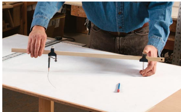
Medium. A beam compass is a two-part drawing tool that attaches to a strip of wood. It can render curves from 1 in. to several feet in diameter.
