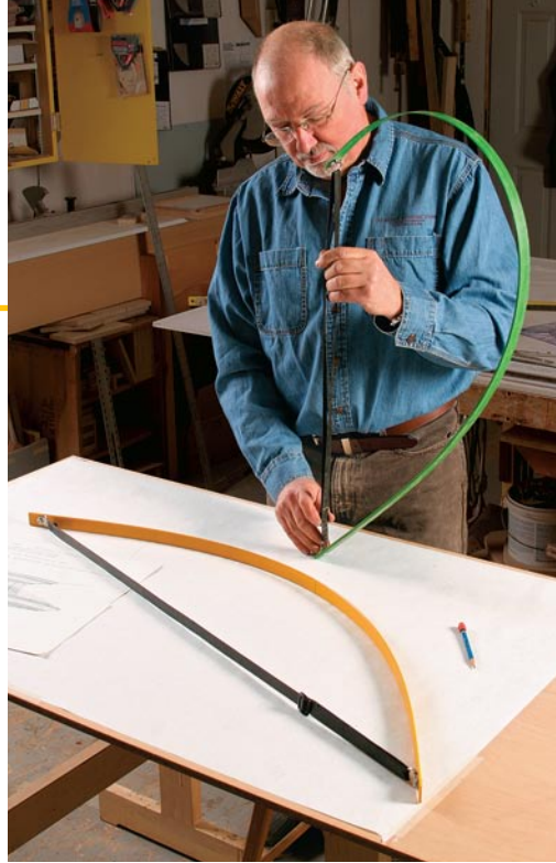
Large. Drawing bows, both symmetrical (yellow) and asymmetrical (green), are bent into shape by tensioning and locking the strap.
