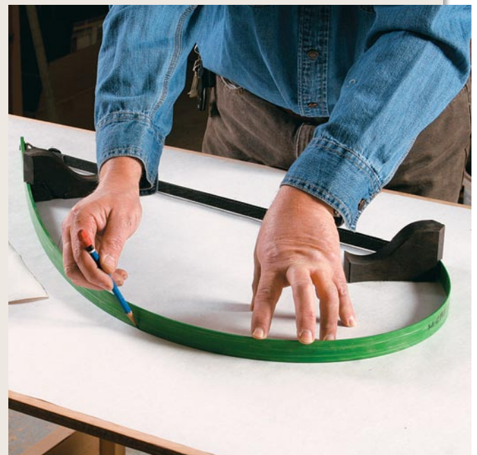
Heavy helping hands. It's tough to hold the bow and trace a line at the same time. If you don't have a helper, use spline weights, often called whales by boatbuilders, to keep the bow still as you scribe the curve.
