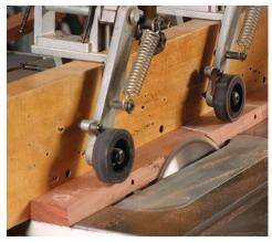
**Bevel the stave.** Set the blade to the angle recorded by the protractor and bevel both sides of each stave to the same angle.
