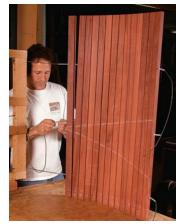
Connect the staves. After feeding the tubing through the holes. stand the staves upright and insert a cable through each tube.
