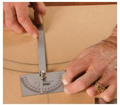
**Calculate the angle.** With the base of a protractor on the pencil line just drawn, swing the arm until it bisects the curve on the centerline and record the angle.
