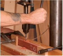
**Precision drilling.** It is critical that each set of holes line up across the staves, so drill the pieces before beveling them. Use a drill press with a fence and a stop block.
