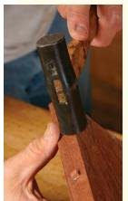
Add outside staves or plug the holes. You can reserve a pair of staves and glue them to the finished panel (above), gluing temporary clamping blocks to the workpiece. Or use a piece of matching wood to create a nearly invisible plug (left).
