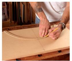
**The right curve.** After creating a pleasing curve and cutting it on a template, transfer the curve to a piece of plywood or MDF and mark the centerline.
