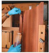
Glue the staves and put the jig to work. Apply the glue using a squeeze bottle and a small brush (above), opening up each pair of staves one at a time. Use a powerful electric drill equipped with a socket to turn the threaded rod (below) and gradually pull the staves together.
