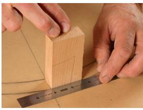
**Work from the center outward.** Use a sample block in place of the unwieldy stave to discover its correct location at the center of the curve. The center of the block should just touch the outside line. Mark this line using a ruler.
