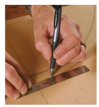
**Mark the line.** Remove the sample block and draw a short line against the edge of the ruler.
