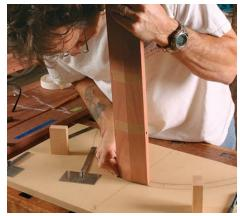
Align the center staves. Tape together the two beveled center staves and place them on the template.
