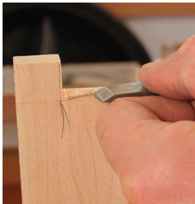
Clean up the corner. The stopped cut will leave a chunk of material on the inside corner, but it's easily pared away with careful chisel work.
