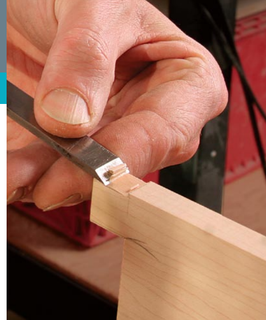
Cut the front shoulder. After defining a \frac{1}{16} -in. shoulder with a handsaw, pare to the line using a chisel.
