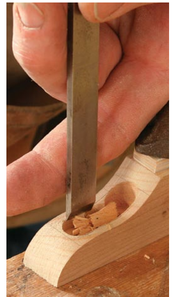
Slotted brackets get special treatment. First use a 1/2-in. Forstner bit to hog out the wide area of the recess that will hold the washer (top left). Use a 3/16-in. bit to rough out the slot (bottom left). Finally, clean up both cuts with a chisel (right).
