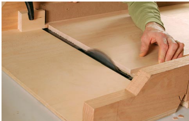
Trim the shelf to form the tenons. Rough out this long notch on the bandsaw. Then clean it up with a stopped cut using a crosscut sled on the tablesaw. Raise the blade high to reduce the amount of waste left near the tenon.
