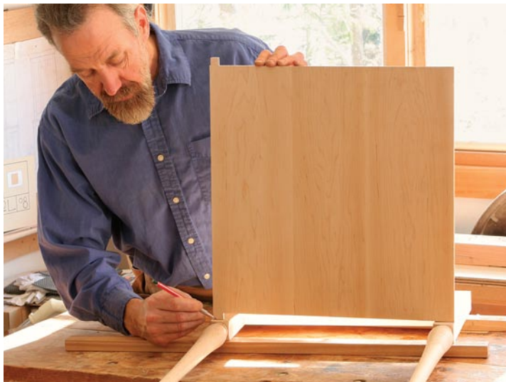
Lay out the mortises. Mark the top edge of the shelf on all four legs. Place the shelf on a front and rear leg and mark the bottom of the shelf on the rear leg. Then mark the mortise for the tenon on the front leg.
