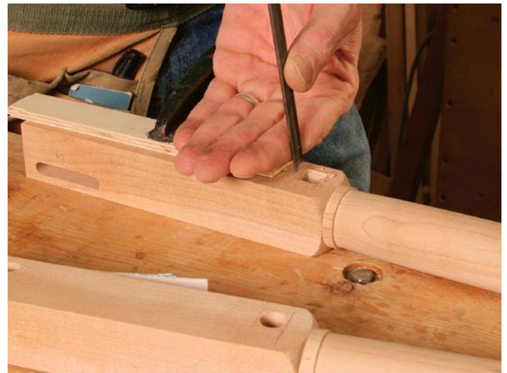
Cut the mortises for the front tenons. Drill out most of the waste, then pare to the line with a chisel. Check the fit often.
