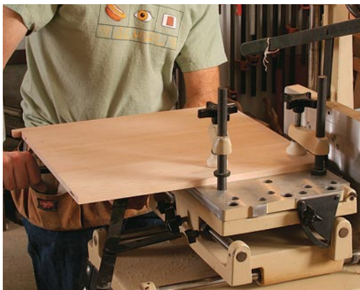
Cut the slots. Turner cuts the narrow slots in both the shelf and legs using a slot mortiser. You could do the same job with a router mortising jig.
