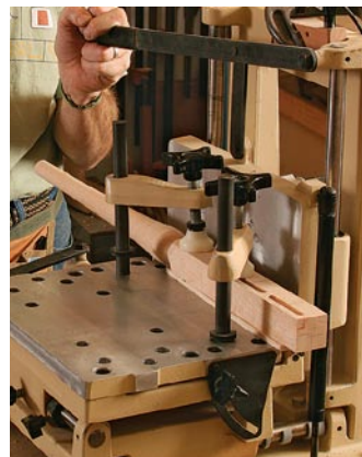
A perfect fit. The loose tenon is glued into the leg but not the shelf.
