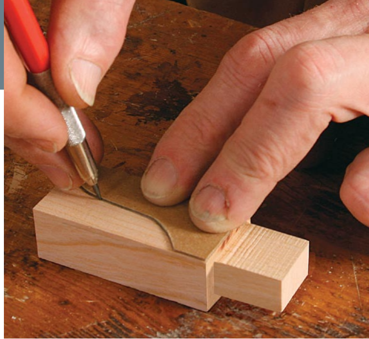
Trace the profile. After cutting the tenons on the bracket blanks, trace the profile using a template and then cut it on the bandsaw.
