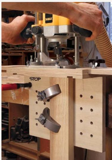
**Into end grain.** The jig is flexible enough to allow end-grain mortises to be cut, such as for slip tenons.
