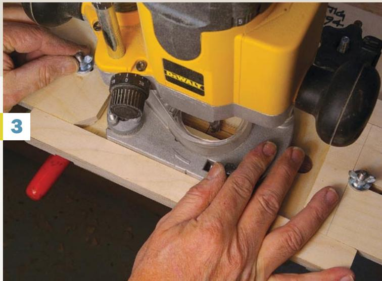
Guide rails and stops are rabbeted to avoid trapping sawdust while routing.
