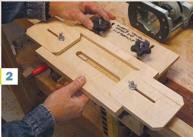
**Adjust front to back and side to side.** Slide the top so the view port is centered on the mortise (above). With the router bit just touching one end of the mortise (right), move the slide until it touches the router base and tighten the wing nut.
