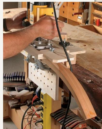
**Curved pieces, too.** The jig allows clean, accurate mortises to be cut on all sorts of curved pieces.
