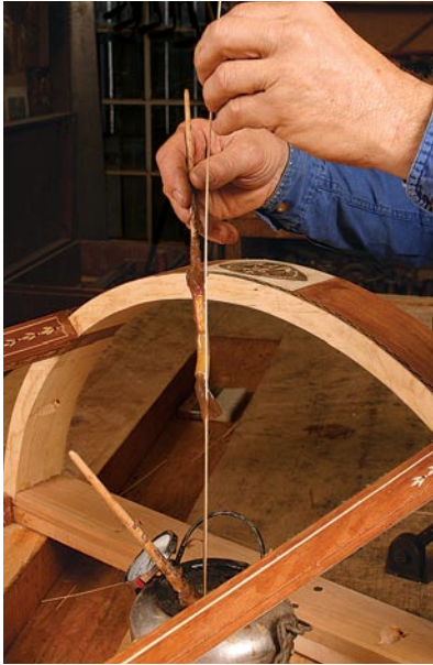
Apply hot glue and press it in place. Be sure the inlay is sized correctly, and then brush glue onto it.
