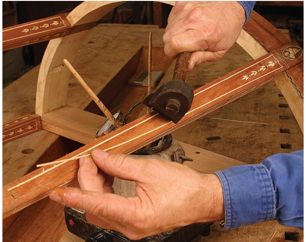
Press it in place. Edwards uses a veneer hammer to push stringing evenly into its groove.
