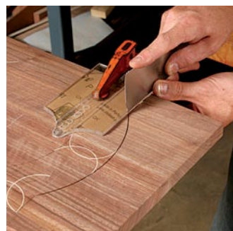
Cut the short segments and clean up the corners. Use the freehand tool against a straight-edge, which is clamped to the surface, to make the grooves straight (above). Use a chisel (right) and a dental pick with a chisel tip to clear debris from the corners. A set of four dental-style carver's cleanup picks is $9.50 from www.leevalley.com .
