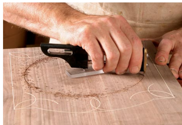
Rotate the workpiece as you cut. This is less awkward than walking around your bench to complete the circle. Be sure that the outer circle cuts through the bottom of the interlaced arcs, creating a seamless transition.
