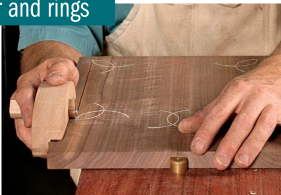
Plow the straight borderlines. The straight-line cutter's fence keeps the blade parallel to the edge. The tool acts as its own depth stop.
