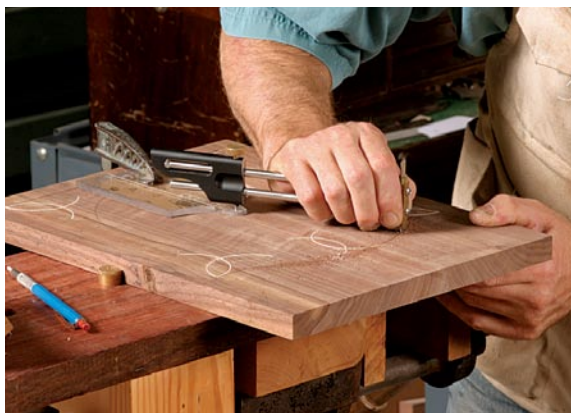
Cut the upper arc. Be sure that the blade cuts through the tops of the interlaced arcs so that they connect seamlessly with the borderline.
