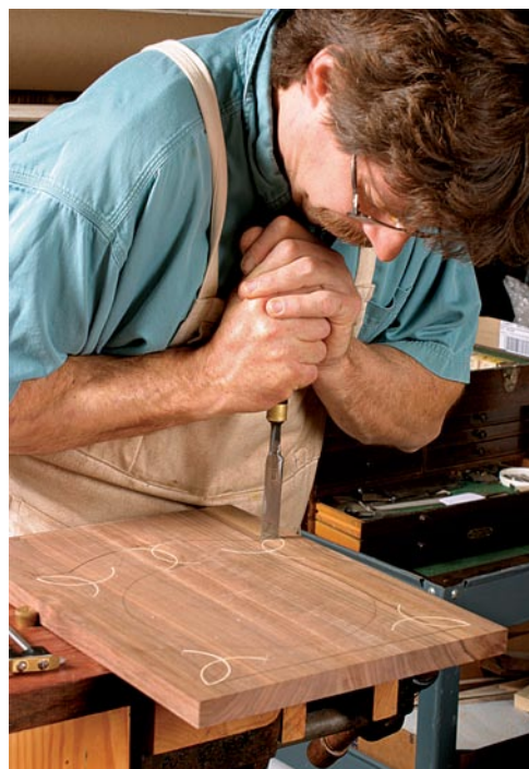
Cut the upper arc. Be sure that the blade cuts through the tops of the interlaced arcs so that they connect seamlessly with the borderline.
