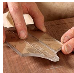
Shield the surface. The centerpoint for this arc won't fall on a future inlay line, so protect the walnut from the cutter's sharp pivot with a piece of Lexan. Drill a hole partially through the plastic to receive the point.
