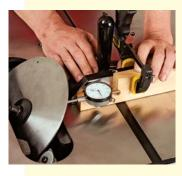
allows the blade to rise up and down and to tilt from 0° to 45°. The Craftsman and Steel City saws have cabinetmounted trunnions, which means the table can be easily and independently adjusted if it isn't parallel to
