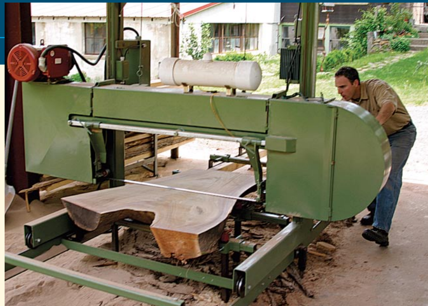
Setting up. Hudock adjusts his bandsaw mill to cut a 2½-in.-thick sycamore slab.
