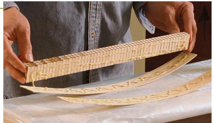
**Veneer the blank.** After planing, glue pieces of  $\frac{1}{16}$ -in.-thick holly veneer to each face.
