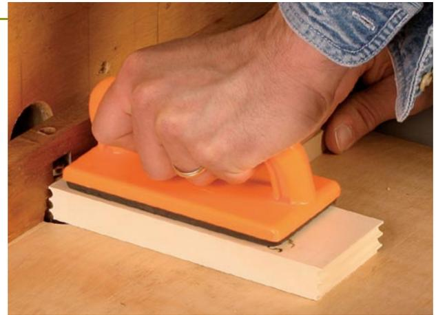
**Route the flutes.** Route the end grain of the holly and the walnut stock using a push block and backing board to control the workpiece and prevent chipout.
