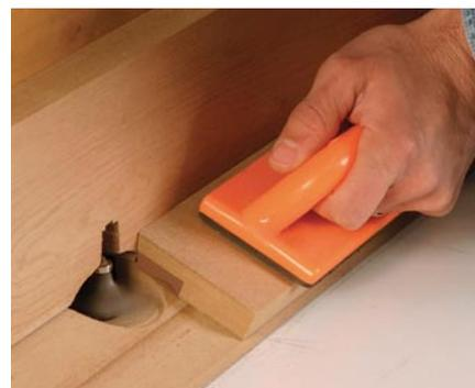
**Use push blocks to keep the work against the fence. If the backer board moves away from the fence during routing, the workpiece will be ruined.**
