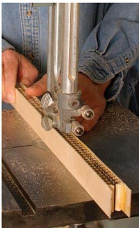
Draw a center-line and make a freehand cut on the bandsaw.
