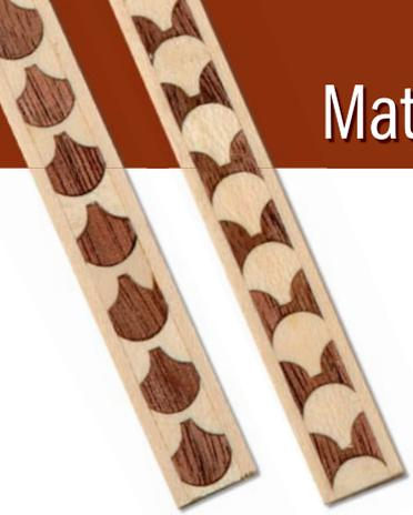
For this banding you'll need two cutters, a beading bit and a fluting bit, whose profiles nest together with the beading bit creating small quirks between the beads.
