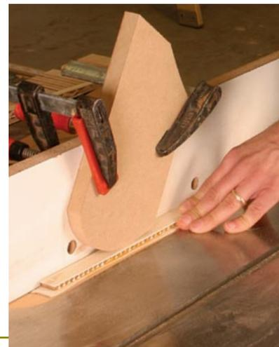
**Rip the bandings.** Arnold uses a thin-kerf blade to rip his bandings to 3/64 in. thick. A piece of MDF acts both as hold-down and blade guard. He pushes the strip as long as is safe, then pulls it from the back side of the blade.
