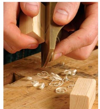
**Create a chamfer.** Using a block plane is the easiest way to chamfer a glue block.
