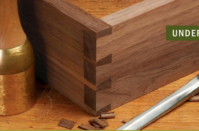
**Good fit where it counts.** As long as the outer edges of the tails and pins are kept clean and tight, the dovetail is aesthetically correct.
