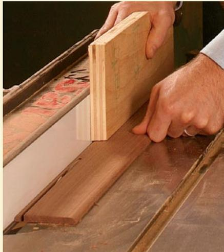
After the profile is cut, rip the molding to thickness with the blade set at 91°.
