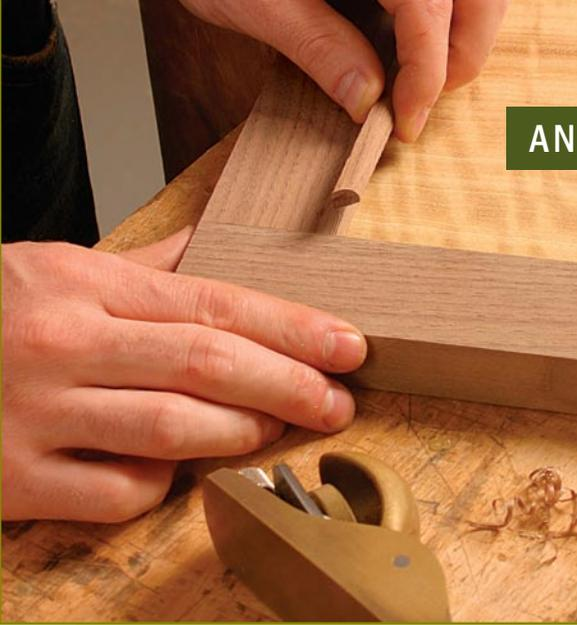
**Easy-fit molding.** Cutting edges at 91° and chamfering the back corner allow for a flawless fit on molding details.
