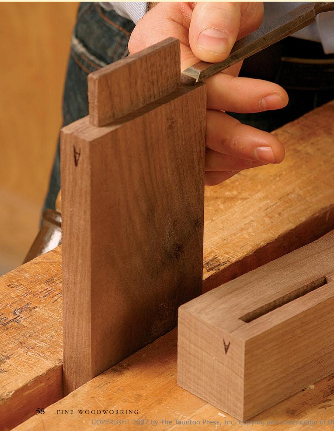
It is a common misconception that fitting a joint means methodically paring the entire area until all the surfaces match perfectly, but in many cases, wood needs to be removed only from hidden surfaces to allow a joint to close completely. I call this technique undercutting.
