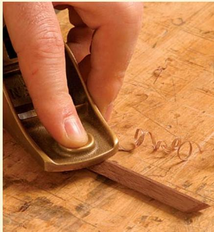
Chamfering the molding's back edge creates additional clearance for a good fit and for hiding glue.
