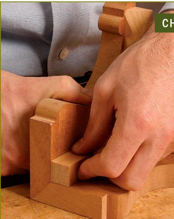
**G**lue blocks are great for adding strength to joints. They can be used to support drawer or chest bottoms, to strengthen bracket feet and mitered joints, and to attach tabletops. However, if there is dried glue squeeze-out in a corner, you won't be able to press the glue block against both sides of the joint. Put a slight chamfer on the inner corner of the glue block, providing clearance for glue or debris.
