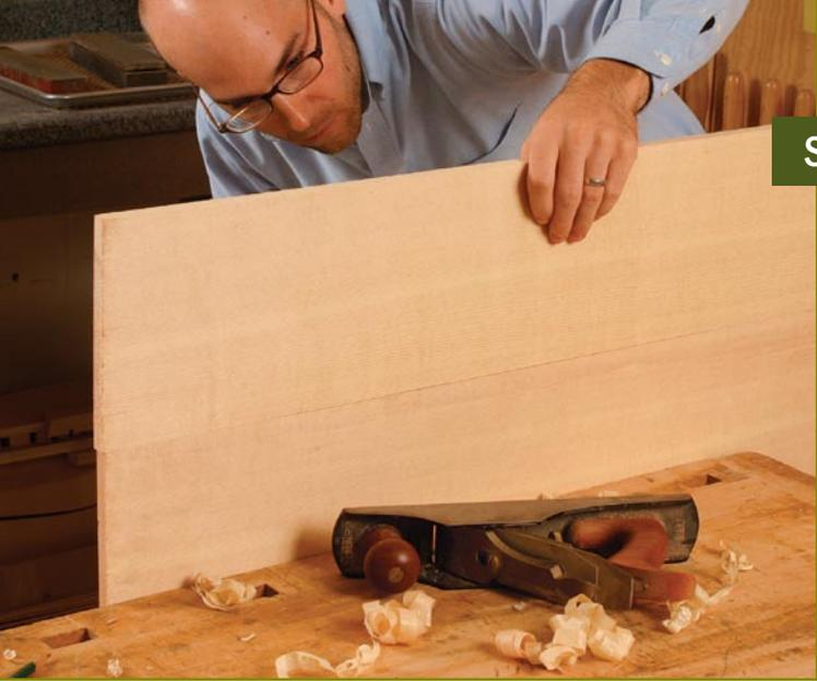
**Bombproof joint.** A nearly imperceptible gap,  $\frac{1}{32}$  in. at most, toward the center of an edge joint ensures a tight fit for decades.
