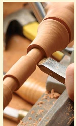
**One-touch technique.** Use a skew chisel to undercut a pull while it is still on the lathe.
