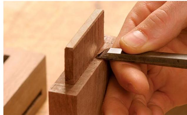
**Carry the bevel around the shoulder.** Work your way around the perimeter of the tenon, leaving the outermost edge intact.
