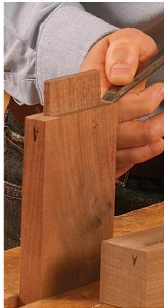
**Undercut tenon shoulders.** Use a chisel to cut a slight downward bevel (no more than 1/32 in.) on the tenon shoulder.
