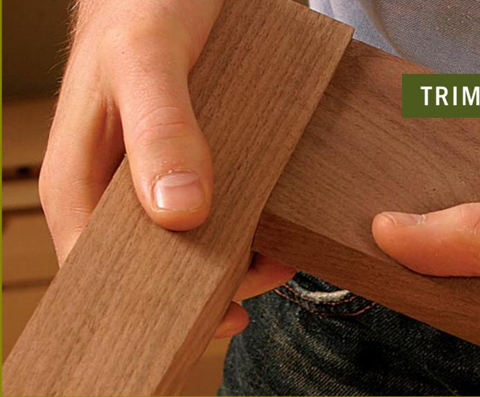
**Gap-free table legs.** Undercutting is an efficient method for improving the fit of a mortise-and-tenon joint.
