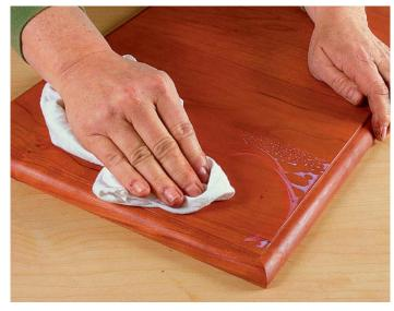
Attack immediately. Wipe off all the contaminated topcoat as soon as you see it crawl. A light spray of shellac will isolate the contamination, so you can reapply the topcoat.
