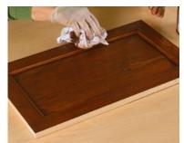
Apply a glaze and wipe it off. Brush on a glaze to help cover up the blotches. Once the excess glaze has been wiped away, the door's color is much more uniform.
