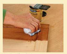
**No blotching.** Stain over a shellac washcoat has much less tendency to blotch.
