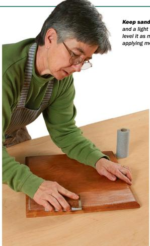
**Keep sanding.** Using fine sandpaper and a light touch, sand the surface to level it as much as possible before applying more topcoat.
