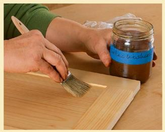
**Control penetration.** A light coat of shellac thinned to a 1-lb. cut creates a good foundation before coloring the wood.
