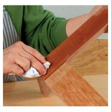
**Solution:** You can get rid of some fingerprints by wet-sanding with the stain you used, or by lightly sanding and reapplying the stain.
