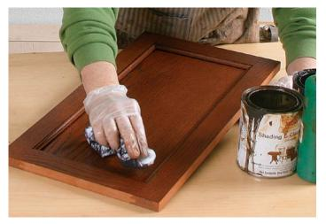
**Solution:** Correct the color with a glaze. I've had good results with Behlen or Mohawk glazing stains. Apply a washcoat of shellac over the stain, then gently scuff-sand with P320-grit paper when it's dry. Use a glaze that contrasts with the stain to bring the color back into line.
