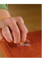
Scrape or sand. Once a drip has dried completely, scrape it off with a razor blade (above) or sand it flush (right).
