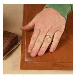
Burned up. If you sand the topcoat too aggressively or don't keep the sanding block level, you risk removing some of the finish.
