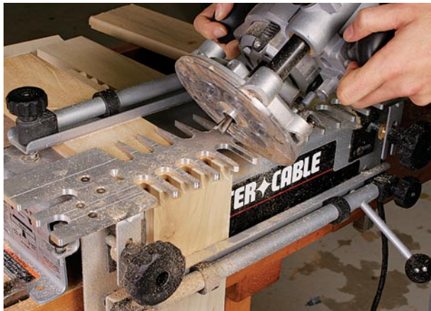
Finished tails. The dovetail bit supplied with the jig cuts the tails. To prevent tearout, use scrap to back up the workpiece.
