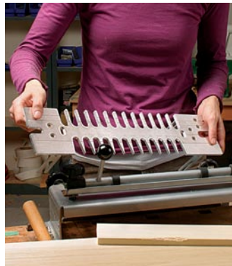
Beginning the pins. Once you've cut tails for all the pieces, you need to flip the template to get ready to cut pins.
