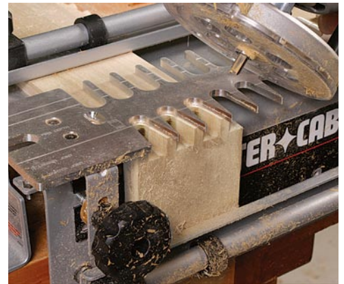
Finished pins. The straight bit supplied with the jig cuts the pins. Here, too, scrap backs up the cut to prevent tearout.
