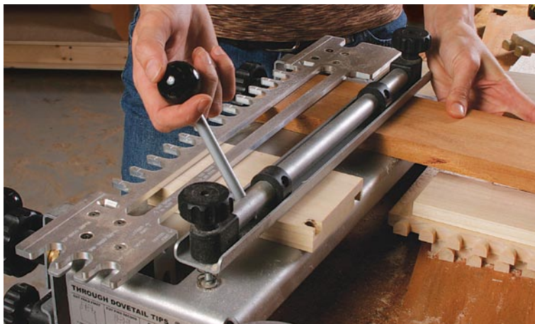
Lock up. Cams on an adjustable locking bar secure the workpiece for the dovetail pins. A piece of scrap the same thickness as the workpiece will keep the jig's template in line.
