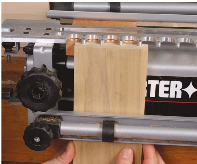
Aligning tails. The same stop that registers the pin board also registers the tail board.
