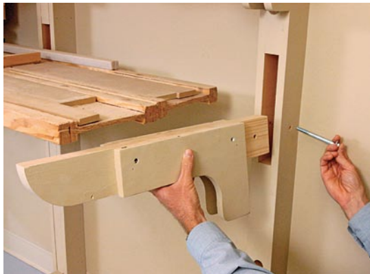
Simple mounting system. Lumber rests on a series of support arms that are bolted to stanchions.
