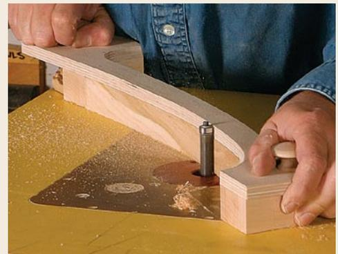
**Quickly clean up the bandsawn edges.** A pattern-routing bit rides along the pattern, trimming the workpiece to its final shape.
