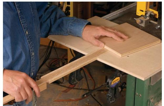
**Attach the stop.** After measuring the distance from the pivot point to the blade (circle radius), clamp the stop on the underside of the arm at the end of the guide track (above left).
