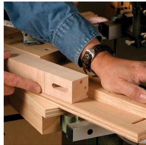
**Locate the taper's start.** Align the beginning of the taper with the edge of the jig and tighten the infeed knob.
