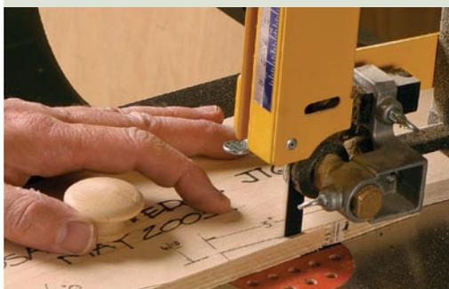
**Cut notches on the jig freehand.** Draw the wedge on the jig, by tracing it or by determining its angle or its length and width. Clearly mark these measurements on the jig.
