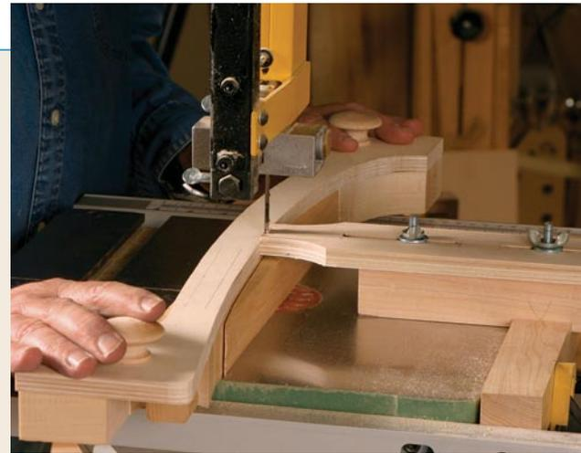
**Raise the finger to cut complex curves.** Adding a block to raise the finger jig, and placing the pattern atop the workpiece, makes it easier to keep the pattern on track.
