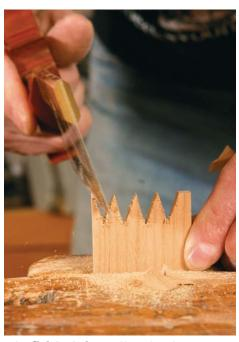
**Mark wider stock than you will need for the finished pieces.** Use a bevel gauge to mark a row of triangular teeth, and then cut the teeth with a dovetail saw.
