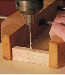
Complete the clasp. Choose the best-fitting teeth and rip both pieces to width on the tablesaw (top). Then clamp the mating pieces together and use a drill press to bore a hole for the pin (left).
