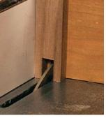
Cut the mortised piece first. Using a block of wood clamped to a miter gauge and the tablesaw fence to support the workpiece, cut the open mortise.
