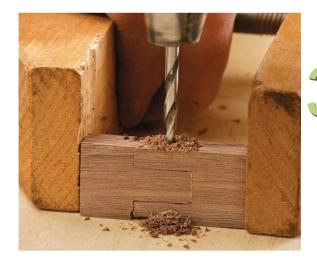
Drill both pieces at once. Clamp the mating pieces together and use a drill press to bore a hole for the pin.
