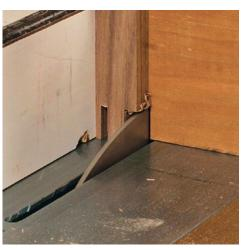
Mark and cut the tenon. Stack the mortised piece on top of the tenon blank, aligning the edges of both pieces. Use a knife to get accurate marks for the tenon (left). Cut the tenon on the tablesaw (right). Adjust the fit as necessary with a chisel and cut both pieces to length.
