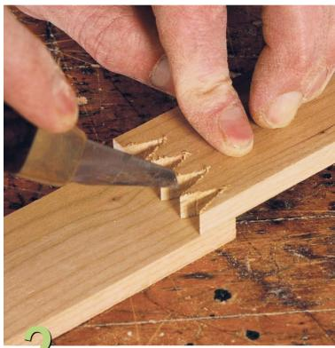
**Mark the matching teeth.** Use the first section as a template for the second, cutting several more teeth than you'll need in the finished clasp.
