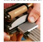
color-coded blade-registration jig engages a slot on the front of the jig body and makes it easy to set a blade not only to the desired honing angle (from 10° to 54°) but also square to the stone. The instructions are well written and easy to comprehend.
