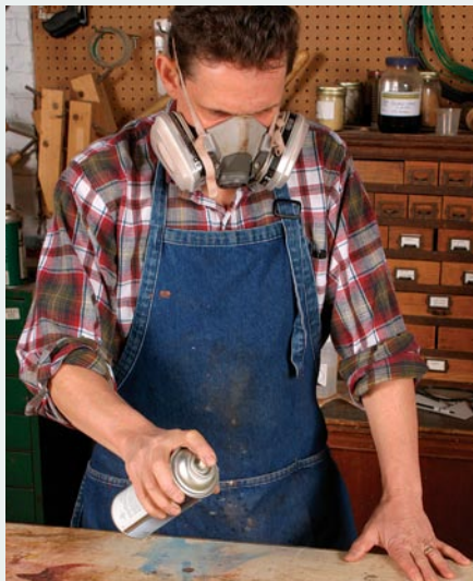
Seal the inlay. Apply several light coats of lacquer to the unmasked banding (left). Then wipe or brush on a dye or stain that won't dissolve the sealer (above).
