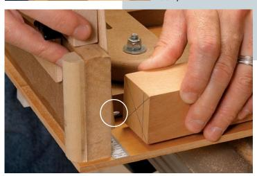
ment that slips over the jig's handle. The pivoting side of the attachment has a nail that engages and supports the leg as it's being tapered. Mark a center point on the bottom of the leg. Use an awl to punch the center point. When rotating the leg for all four tapers, it will revolve around this point.
