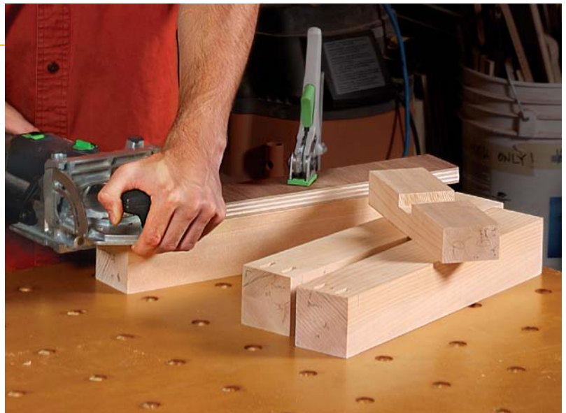
Mortise for the slip tenons. In Wickham's shop, they use a Festool Domino Joiner for the job, but you could use a router or hollow-chisel mortiser.
