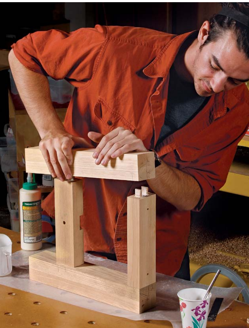
Glue up the end assemblies. Because this bench is for the outdoors, use a waterproof glue. Wickham prefers Titebond III. After assembling the legs and rails, clamp and let the glue dry.
