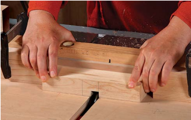
Cut a dado for the long stretcher. Use a stop at both ends of the stretcher to ensure that the dado in each rail is the same width and in the same location.
