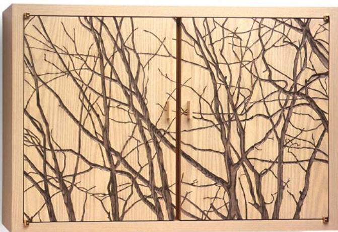
Flowing frame. With the powerful tenons hidden, Gowdy's mitered case works as a clean, elegant border for his carved doors.
