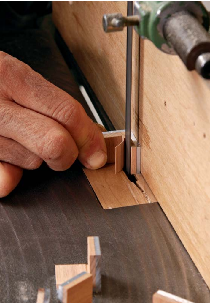
Tenon trimming. Coleman trims the tenon to exact thickness by shaving the wood face on the bandsaw.
