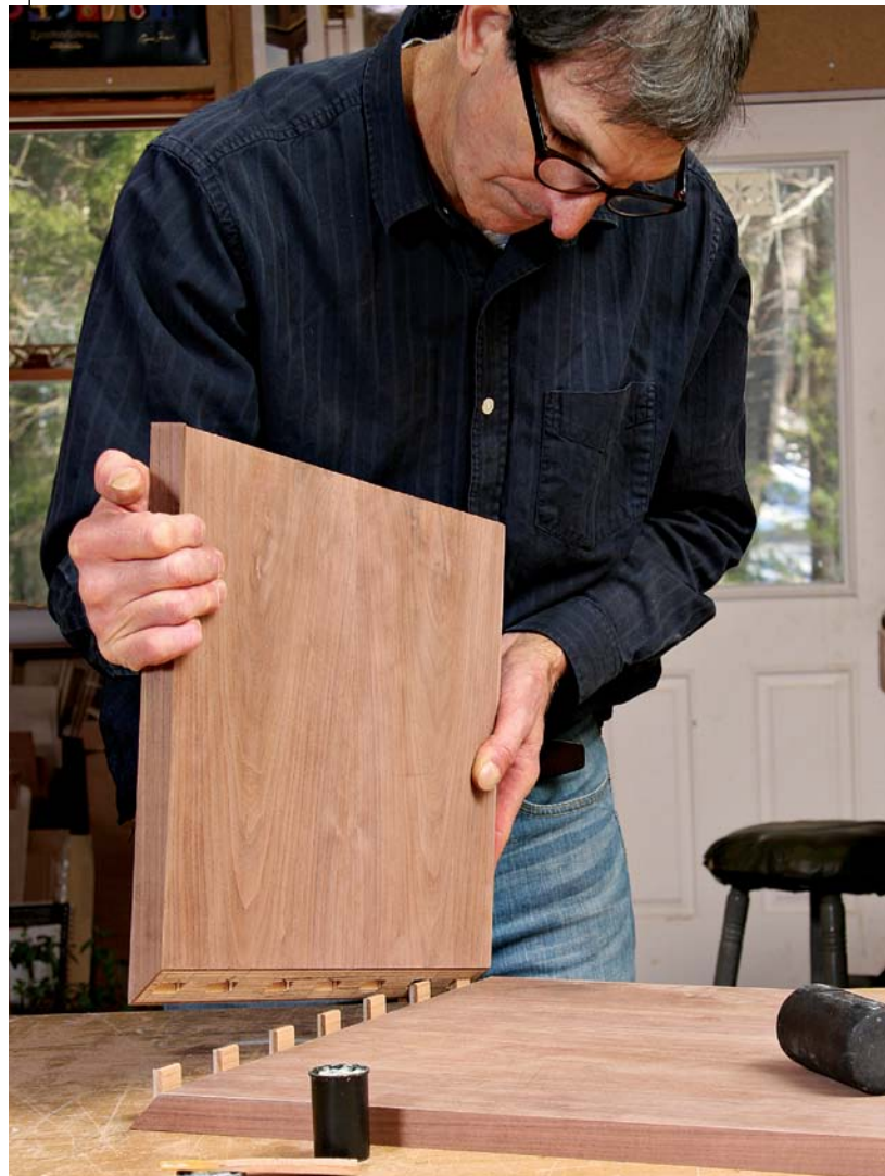
Two-step glue-up. Coleman glues his tenons into one side of the case and lets them dry, then glues them into the second side. This means that to close the joint he needs clamping pressure in only one direction.
