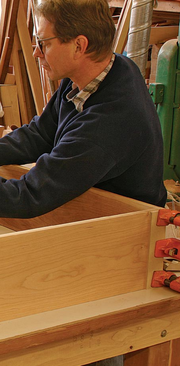
Use melamine cauls and check the diagonals. On dovetails, Rogowski keeps the long grain proud, which allows him to use flat cauls. Later, he planes the sides flush with the pins and tails. If the diagonals don't match, use a long clamp to draw the assembly square.
