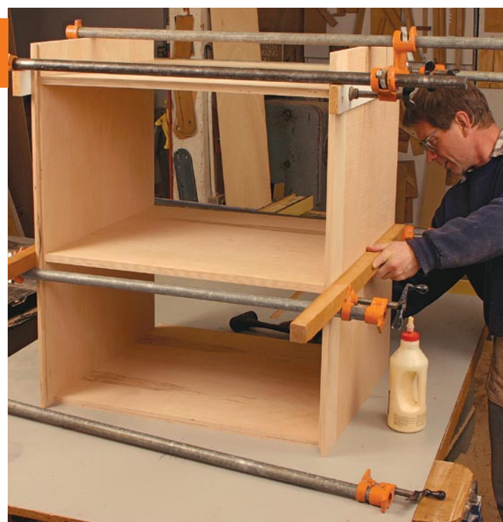
Glue large cases in stages. Here the case is upside down, and the top panel is only dry-fit in its rabbet, while the other panels are glued. To apply pressure along the entire edge of the middle shelf, Rogowski uses a convex caul.
