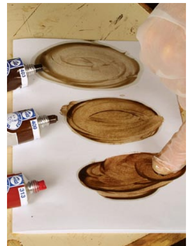
A shopmade glaze. You can make oil-based glaze using boiled linseed oil, gel varnish, and artist's oil colors (left). To check the color and translucency of the glaze as you add artist's oil colors, smear samples onto white paper.
