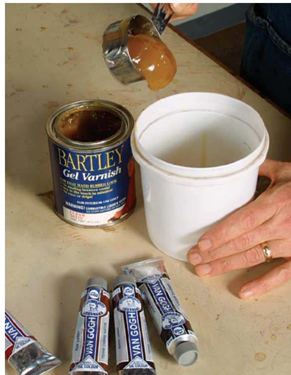
A shopmade glaze. You can make oil-based glaze using boiled linseed oil, gel varnish, and artist's oil colors (left). To check the color and translucency of the glaze as you add artist's oil colors, smear samples onto white paper.
