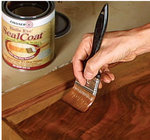
Seal the dye with shellac. After the dye has dried, brush on a thin coat of dewaxed shellac such as Zinsser's SealCoat.
