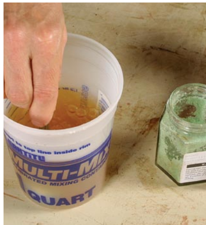
Ferrous sulfate. Also known as copperas, this chemical turns most woods various shades of gray.
