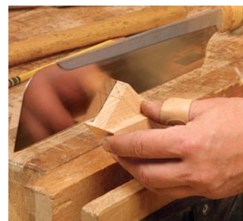
Cut the tenon cheeks first. Use a handsaw, cutting right to the layout lines.
