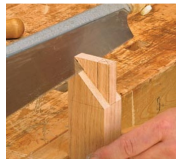
Lay out and saw the last two sides of the tenon. Then saw a little shy of the mitered face to remove the waste.
