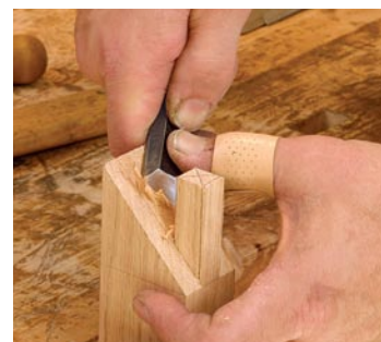
Finish the mitered faces with a chisel. Pare away the small step left behind from sawing.
