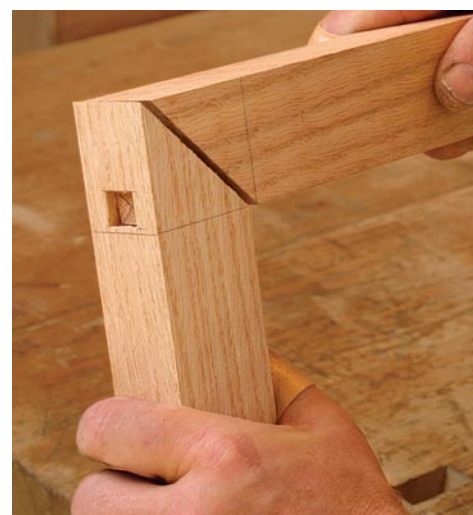
Finish the mitered faces with a chisel. Pare away the small step left behind from sawing.
