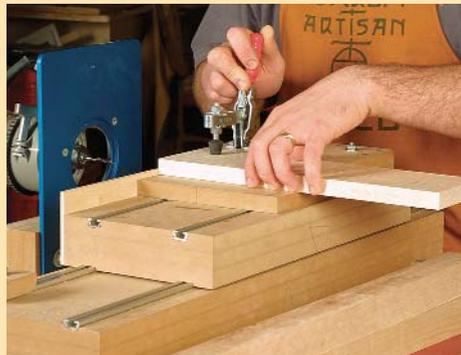
**Clamp the apron to the sliding platforms.** Set the mortise height with a spacer. Then butt the workpiece against the fence and index block, and clamp it in place.
