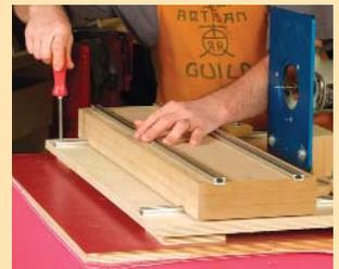
The movable platforms don't make contact with one another; instead, they slide solely on the aluminum T-tracks. The tracks also secure the clamping blocks. Wax the tracks regularly to ensure smooth movement.
