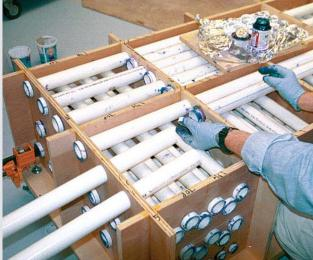
**Install the pipes.** Use PVC glue to attach the rings to the pipes. Work from the lowest row to the top.
