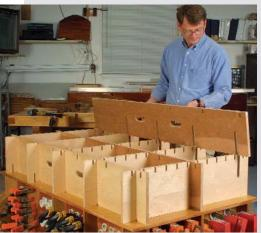
Crosslap joints make for easy assembly and disassembly of plywood grid. Bar clamps rest in grooves cut into the top edges of the plywood grid. The bars extend 1/8 in. above the plywood edge to provide clearance during glue-up.
