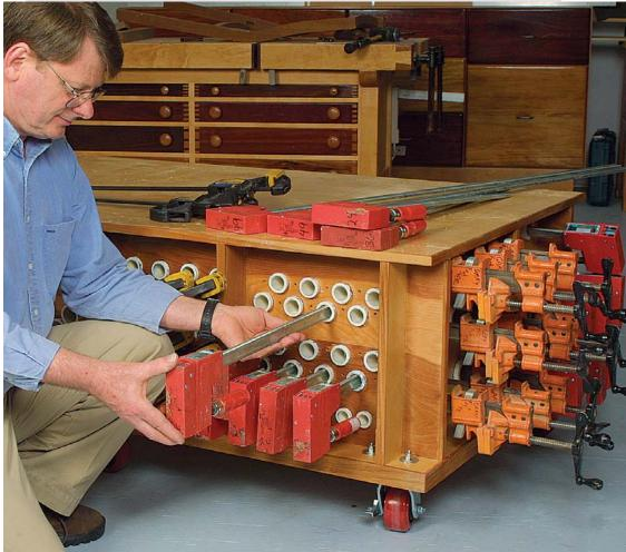
**Space-saving clamp storage.** Offset the holes for the PVC pipes to maximize storage space. If clamps interfere with each other, you can insert some from the other side.
