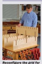
two-directional clamping. Grooves of various depths, cut into the five short plywood panels, allow the grid to be arranged so that clamps situated front to back can sit below those running side to side.
