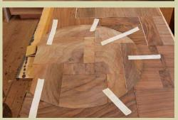
Fitting the circle. After applying a bead of glue around the perimeter of the recess, Hernandez pressed the circle in place. Masking tape stretched across the seams provides the clamping pressure, as seen in the glue-up of the larger circle (left).
