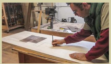
**Full-scale layout** guides the process. After developing a small version of the parquetry pattern on paper, Hernandez roughed it out full-scale on the plywood substrate itself (above), and then drew a fully detailed version on a sheet of 1/4-in. MDF (right), which he used throughout the fitting process.
