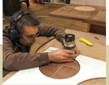
Quick, clean circle. Using the same template and bushing with the wide rub collar removed, Hernandez routed the circular insert.
