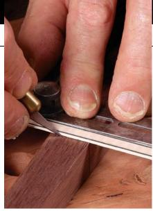
**The banding sets the width.** Use a piece of banding to space the bevel gauge from the first line, then knife the second line.
