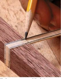
Work your way around the leg. Dry-fit the taped banding in the dado and mark the next joint's location, then miter the next corner.
