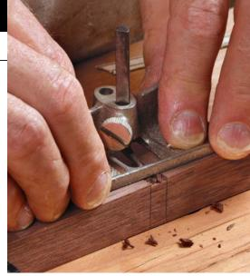
**Finish it with a router plane.** After setting the blade depth by placing cuff banding under the base, clean up the bottom of the dado.
