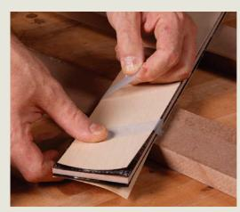
**Bandings start as a sandwich.** Stack layers of veneer and thin-milled solid wood for gluing. Use tape to keep them aligned (above), wrapping diagonally to prevent tearing the grain during removal. Then clamp the stack in the press (right).
