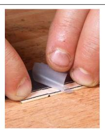
Tape the corners together. Cut thefirst side to length, then line it upagainst a straightedge with the nextpiece, and tape the miters together.
