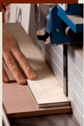
**Ready to rip.** After the banding dries, joint an edge and rip it into <sup>3</sup>/<sub>64</sub>-in.-wide strips using the fence on the bandsaw. You can reduce tearout by using a zero-clearance deck—make one by cutting a few inches into a piece of <sup>1</sup>/<sub>2</sub>-in.-thick MDF, and clamping it to the bandsaw table.
