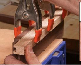
Fold back the banding to put on the glue. The tape acts like a hinge, allowing the banding to fold open for the glue (left), then fold right back into place for a perfect fit. After adding the glue, Latta puts on the clamps with a special U-shaped caul that directs the pressure to the banding (below).
