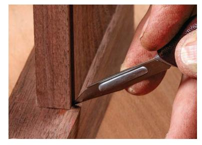
Mark the waist banding on the legs. The waist banding wraps around the aprons and legs at the same height. To ensure that each part meets perfectly, dry-fit the aprons to the legs before transferring the rabbet location to the legs. Then cut the dadoes for the waist banding using the same technique as for the cuff banding.
