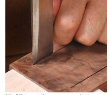
It's OK to cut these corners. Latta uses a 1-in.-wide chisel to establish clean edges near the corners.
