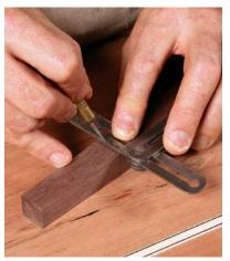
Mark the first line. Measure 2<sup>3</sup>/<sub>4</sub> in. from the bottom of the leg, then use the bevel gauge and knife to mark a line around all four sides.
