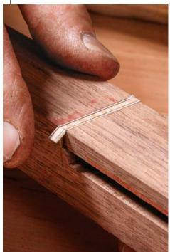
Install the waist banding on the back legs. The banding is mitered around three corners of the back legs. It won't be visible inside the frame, so it stops at the mortises.
