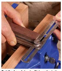
**Set the bevel gauge.** Pick up the leg's taper angle by pressing the bevel gauge against the bottom and side of the leg, then use it to lay out the cuff banding.
