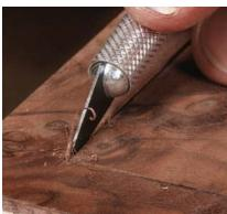
**Turn a hobby knife into a tiny chisel.** Regrind and sharpen an X-Acto knife with square edges and a chisel tip— it's the perfect tool for cleaning out the grooves.
