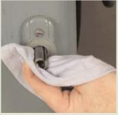
Out with the old. Clean and lubricate all of the parts, then slide a new key into place, which should eliminate any slop in the adjustment.
