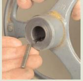
**Pull things apart.** With the handle removed, you see that the key that locks the handle to the adjusting rod has worn out.
