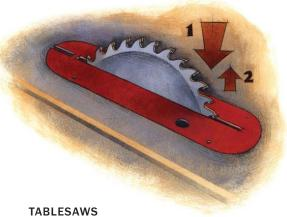
When working at a tablesaw, adjust the blade by raising the arbor assembly to the desired height instead of lowering it. If you need to lower the blade, lower it more than necessary, then raise it to final height.
