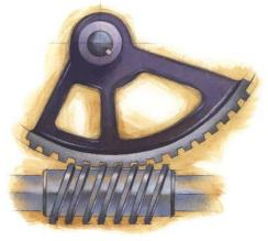
**WORN GEAR TEETH** Rotation of the worn gear pushes against the gear segment, causing the two parts to wear over time, creating more dead space and backlash.
