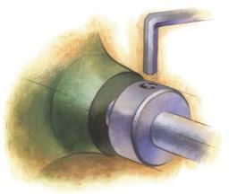
LOOSE COLLARS The vibration caused by normal wear and tear on machines can cause setscrews to rattle loose.
