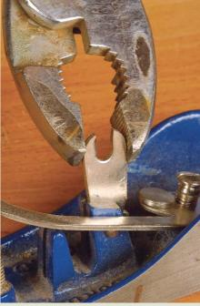
**Reduce the gap.** Close up the slot on the adjuster with a pair of pliers or vise grips.
