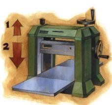
**BENCHTOP PLANERS** The carriage should be lowered into the cut so that the pressure is against the thread on the adjuster.
