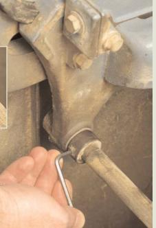
that chain to transfer motion, the links must be in tension. Motion applied to a crank transfers power when all mechanical links are pulled tight; until then you are just taking up slack.
