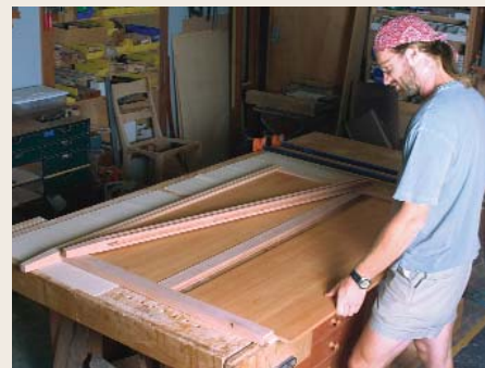
Assemble the back. The two back panels are slipped into the grooves in the frame parts and then clamped.
