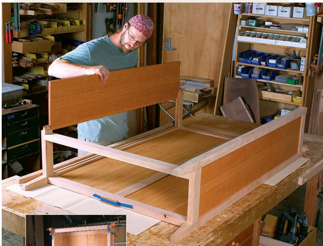
Add the remaining frame-and-panel parts. Once the back glue-up has dried, the remaining frame-and-panel parts are added in one big glue-up. First, the lower front rail is assembled to the two lower side rails, and then all four of the side rails are added to the back posts. Following in quick succession are the side panels, front posts and the upper rail (above). An assortment of clamps keeps the joints tight until the glue sets up (left).
