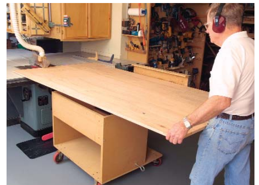
The L-shaped tilting top holds several sheets of plywood. A pin locks the tabletop in the horizontal position. Large locking casters can handle bumps in the concrete without stalling. Pillow blocks make for a smooth pivoting action.
