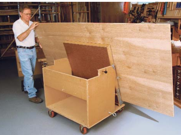
The L-shaped tilting top holds several sheets of plywood. A pin locks the tabletop in the horizontal position. Large locking casters can handle bumps in the concrete without stalling. Pillow blocks make for a smooth pivoting action.
