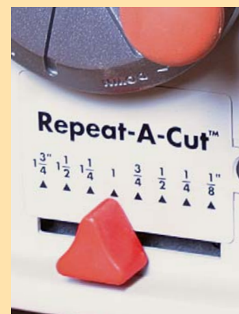
Gauge shows depth of cut. Some of the planers feature a gadget that quickly lets you see how much stock the next cut is going to remove.
