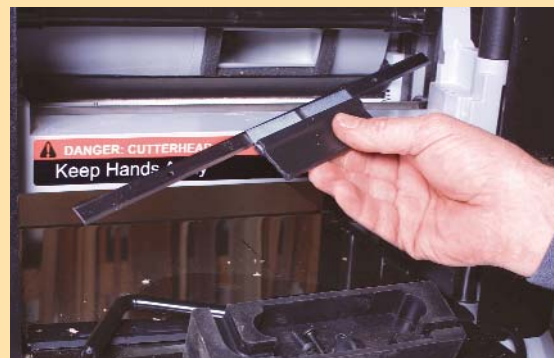
Changing knives shouldn't be a chore. Depending on the machine, the job can take anywhere from five to 25 minutes.
