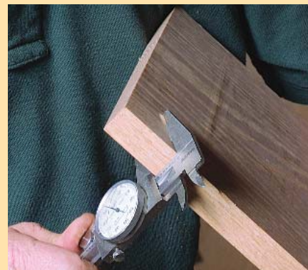
Snooping for snipe. Snipe was measured with a dial indicator.
