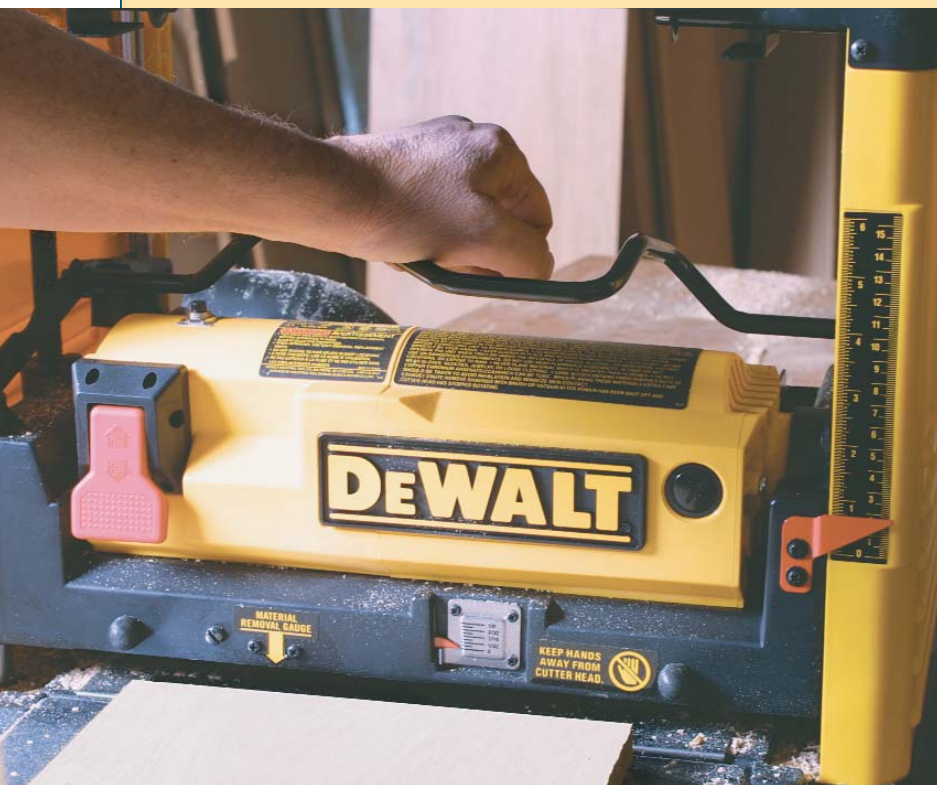
Cutterhead lock helps reduce snipe. In general, the planers with cutterhead locks produce less snipe than those without the mechanism.
